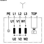
Note: Direction of rotation changes when two phases are reversed
