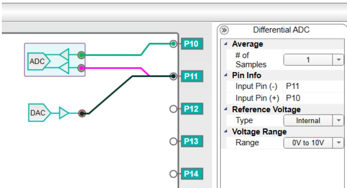
**Figure 10. ADC with Pseudo-Differential Input Set by DAC**
