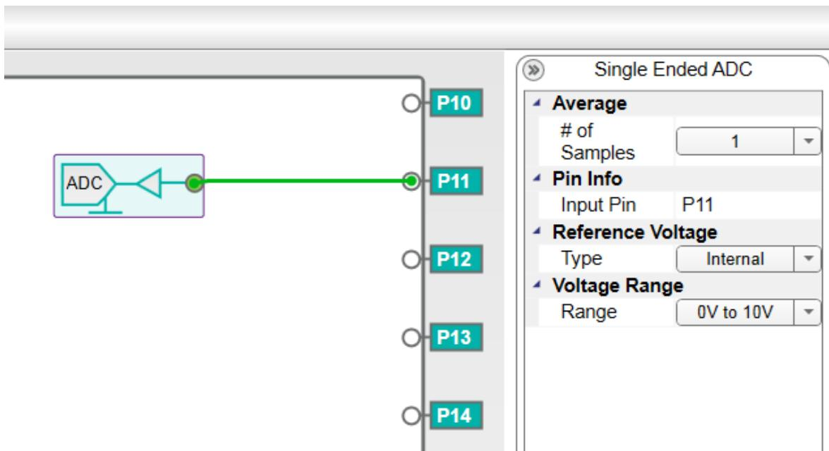
**Figure 8. ADC with Single-Ended Input**
