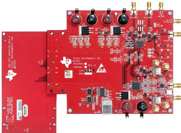
The FMC-DAC-Adapter passive interconnect board enables the output of TI's LVDS input high speed DACs to be directly connected to a standard FMC interconnect header, a typical input on the latest Xilinx FPGA EVMs. This enables users of TI's high speed DAC EVMs to directly interface to Xilinx FPGA's for prototyping purposes, saving the time and cost of producing a custom prototyping board.
