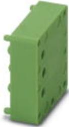
PCB terminal block, Nominal current: 24 A, Nom. voltage: 400 V, Pitch: 5 mm, Number of positions: 1, Connection method: Spring-cage connection, Mounting: Soldering, Conductor/PCB connection direction: 90 °
