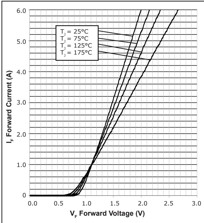
Figure 1. Forward Characteristics
