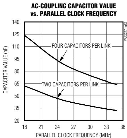
Figure 12. AC-Coupling Capacitor Values vs. Clock Frequency of 18MHz to 35MHz
