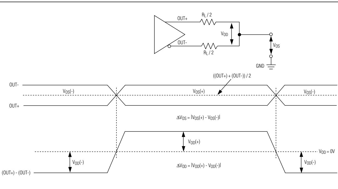
Figure 1. LVDS DC Output Load and Parameters
