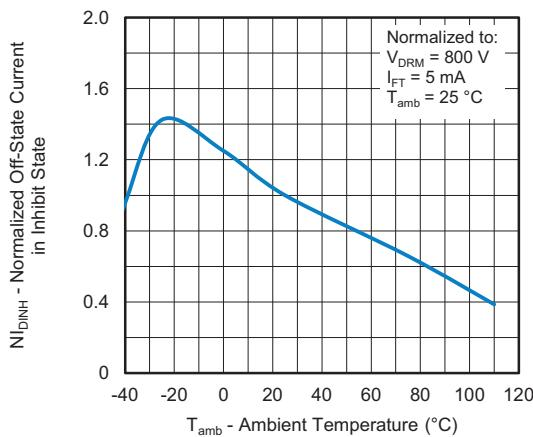
Fig. 9 - Normalized Off-State Current in Inhibit State vs.
