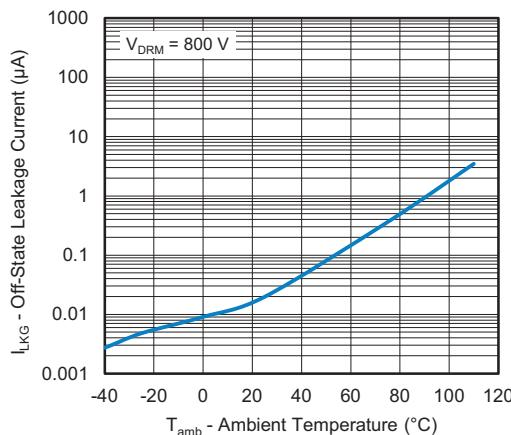
Fig. 8 - Off-State Leakage Current vs. Ambient Temperature
