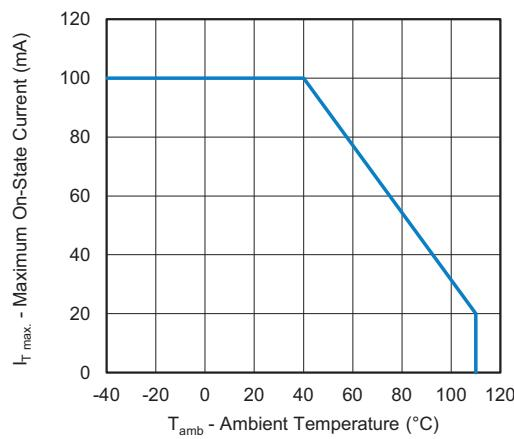
Fig. 2 - Maximum Forward Current vs. Ambient Temperature
