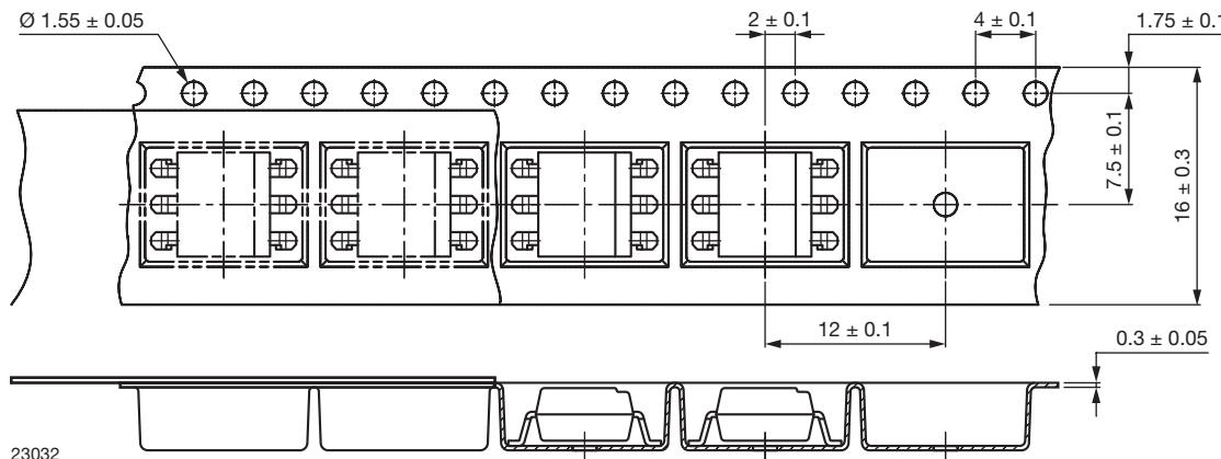
Fig. 17 - Tape and Reel Packaging (1000 pieces on reel)
