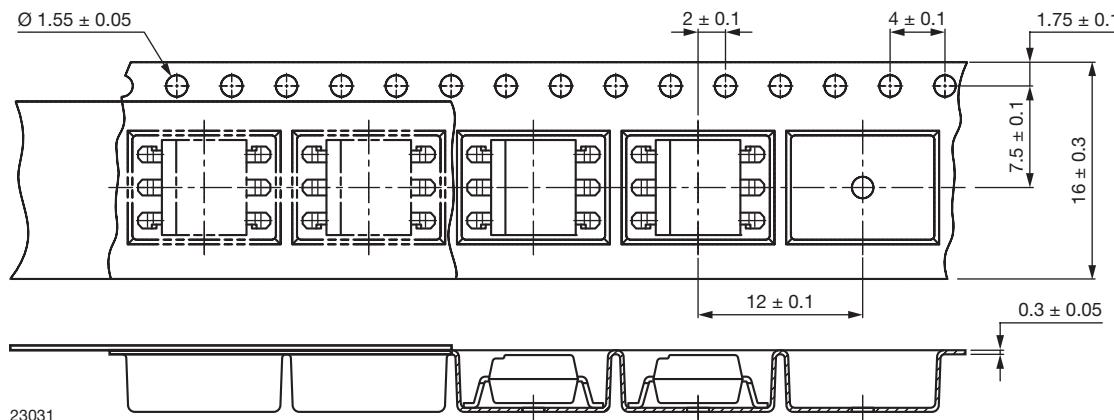
Fig. 16 - Tape and Reel Packaging (1000 pieces on reel)
