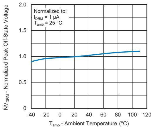
Fig. 10 - Normalized Peak Off-State Voltage vs.
