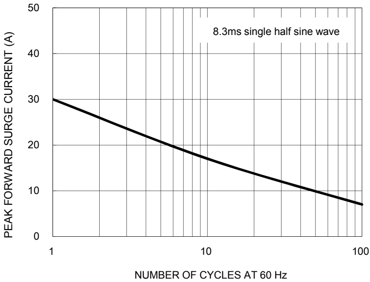
FIG. 3 MAXIMUM NON-REPETITIVE FORWARD SURGE CURRENT
