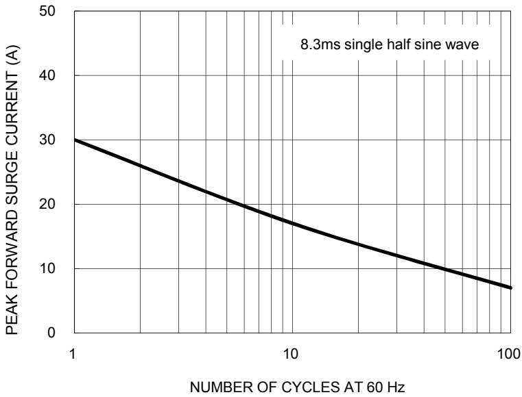
FIG. 3 MAXIMUM NON-REPETITIVE FORWARD SURGE CURRENT
