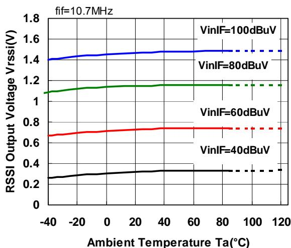
**RSSI Output versus Temperature-50MHz-**
