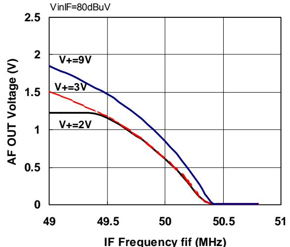
Demodulated Signal Frequency Characteristics
