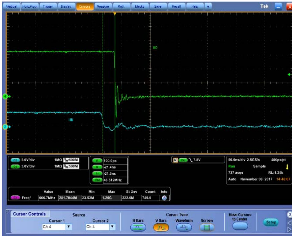
Figure 33. High Side Turn-Off Propagation Delay (NCP51530B)
