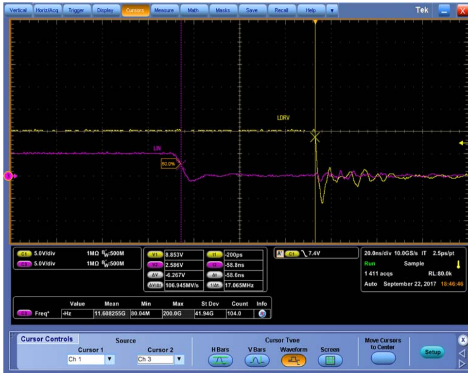
Figure 31. Low Side Turn-Off Propagation Delay (NCP51530A)
