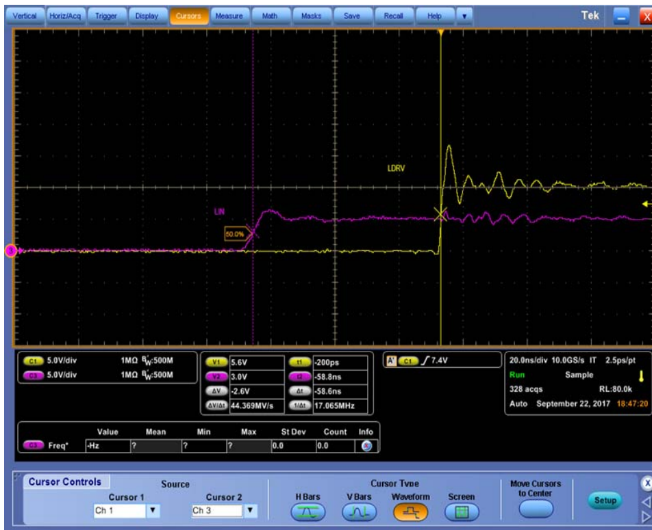
Figure 30. Low Side Turn-ON Propagation Delay (NCP51530A)
