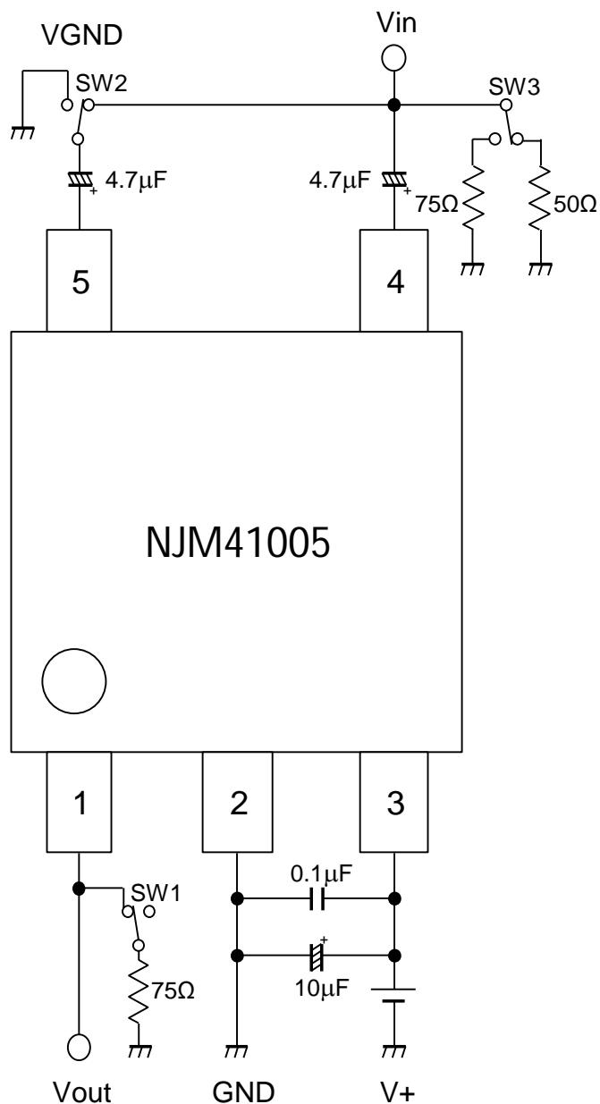
**■APPLICATION CIRCUIT 1**(Output DC Coupling)
