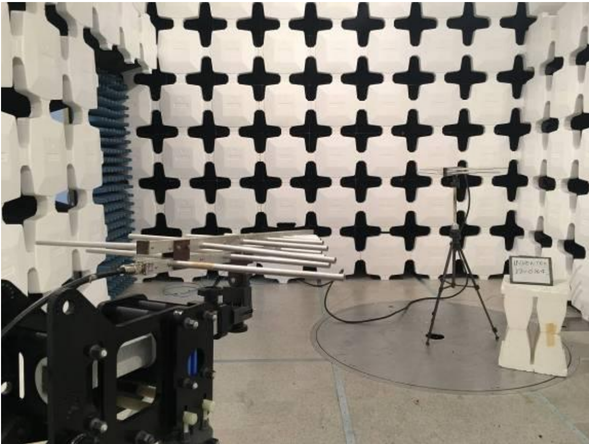
Figure 33. 200-1000 MHz Substitution Testing
