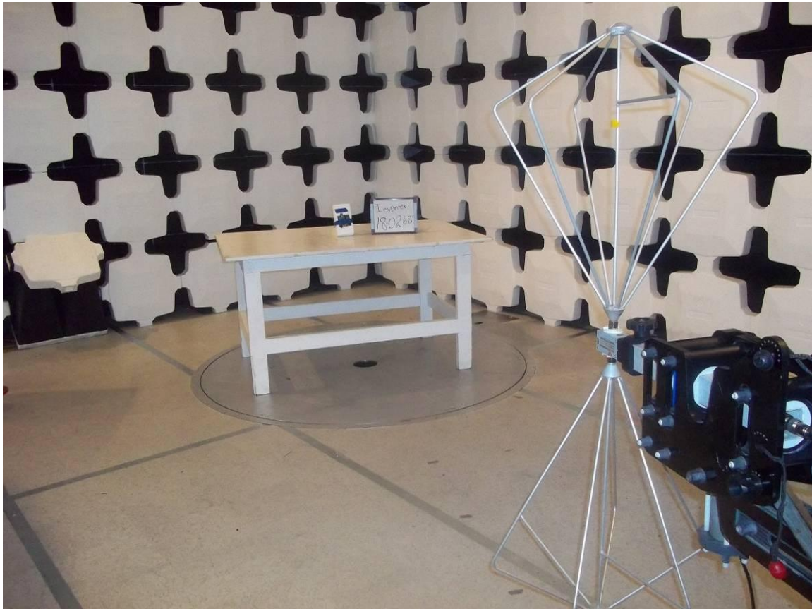
Figure 29. Radiated Spurious Emissions Below 200 MHz
