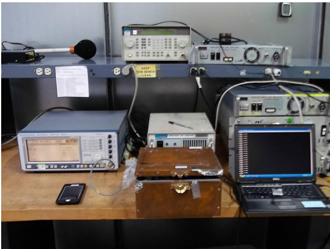
Figure 37. Receiver Blocking Test Setup
