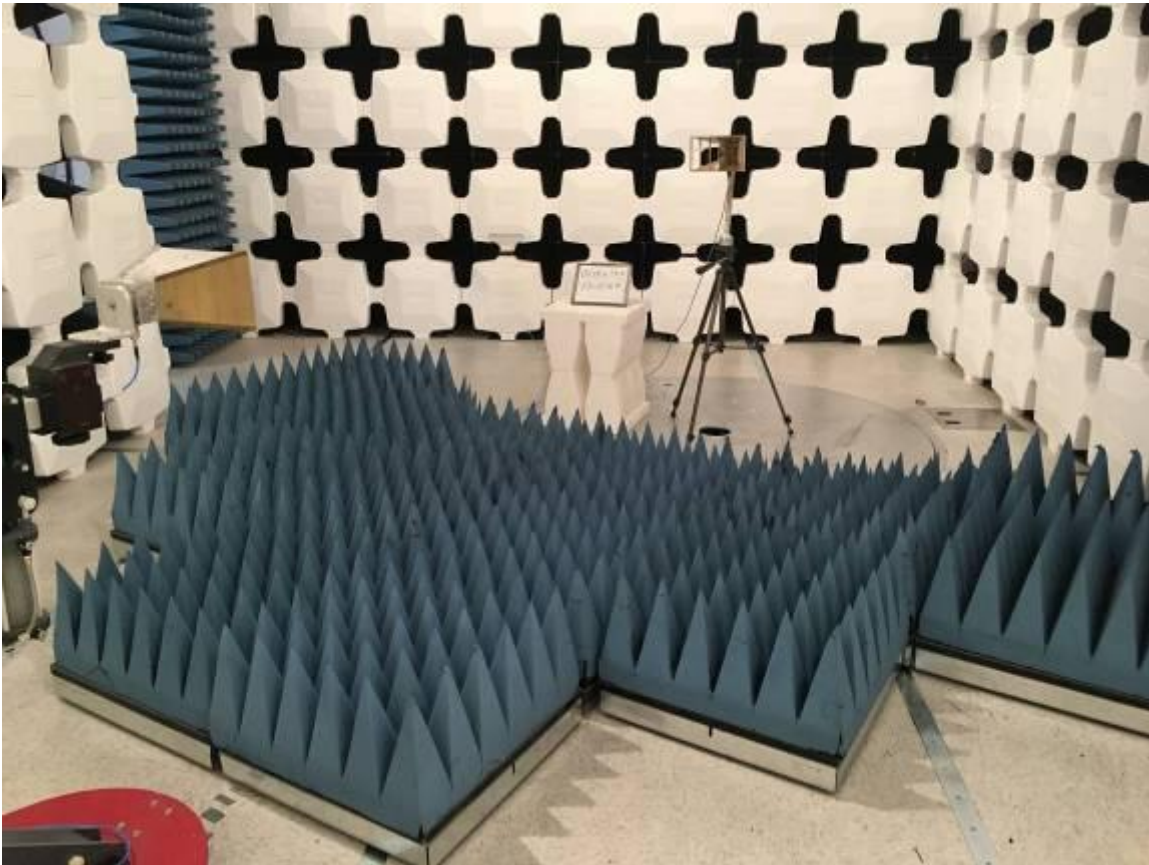
Figure 34. Above 1 GHz Substitution Testing
