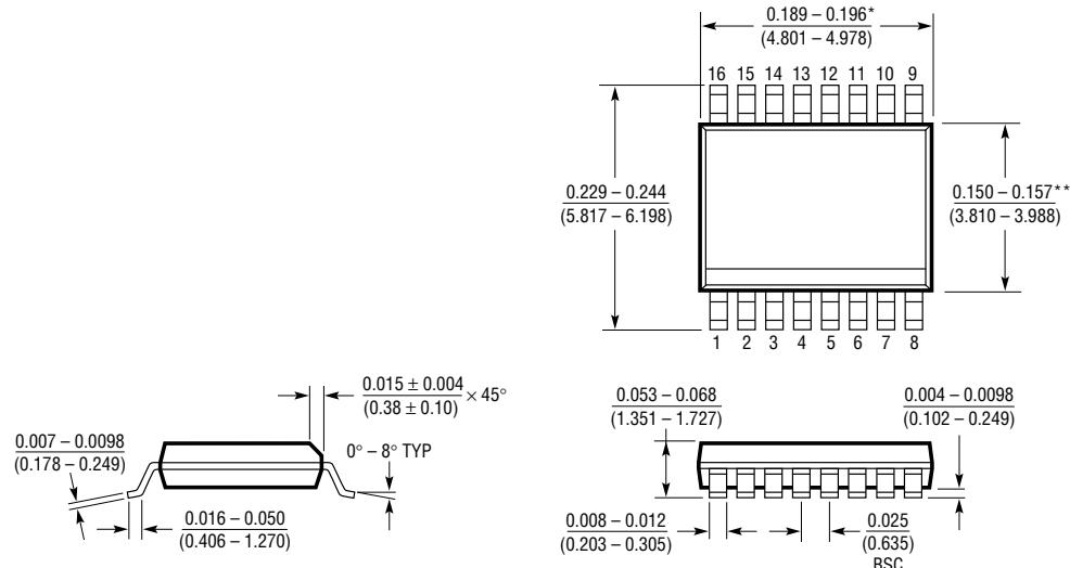
\* DIMENSION DOES NOT INCLUDE MOLD FLASH. MOLD FLASH SHALL NOT EXCEED 0.006" (0.152mm) PER SIDE
