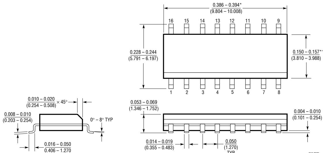
\* DIMENSION DOES NOT INCLUDE MOLD FLASH. MOLD FLASH SHALL NOT EXCEED 0.006" (0.152mm) PER SIDE
