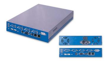
Enclosed in a 1U small box structure, the physical appearance of the BBS-2002 may seem to be identical to a high-powered DC power supply, but do not let its physical attributes mislead you. This small box houses a semi-functional system based on the HS-5230CF PCI-ISA Bus SBC that supports a Cyrix Geode GX1 300MHz low power embedded CPU.
