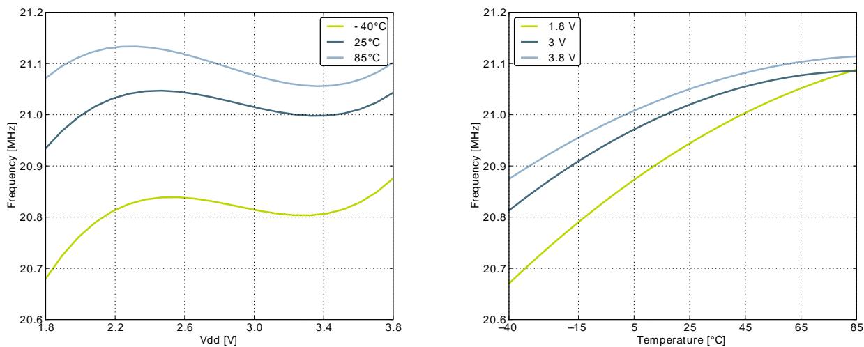
**Figure 3.24. Calibrated HFRCO 28 MHz Band Frequency vs Supply Voltage and Temperature**
