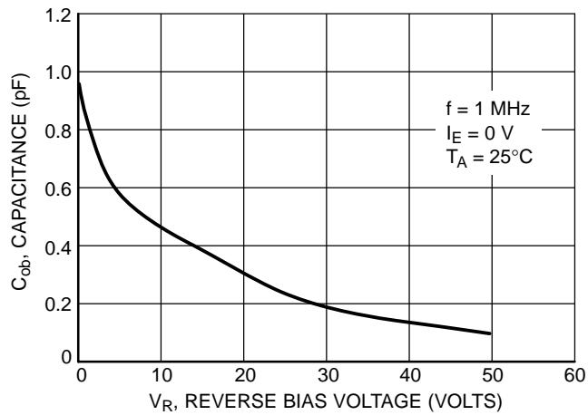
**Figure 35. Output Capacitance**
