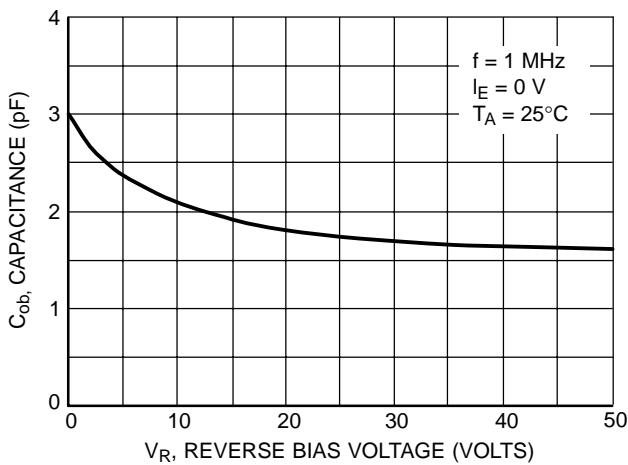
Figure 10. Output Capacitance
