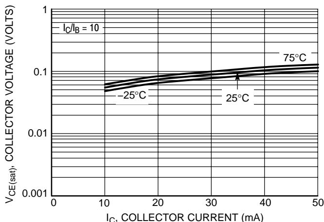
Figure 28.  $V_{CE(\text{sat})}$  versus  $I_C$
