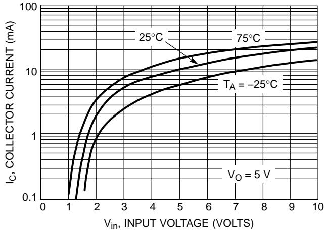
**Figure 36. Output Current vs. Input Voltage**
