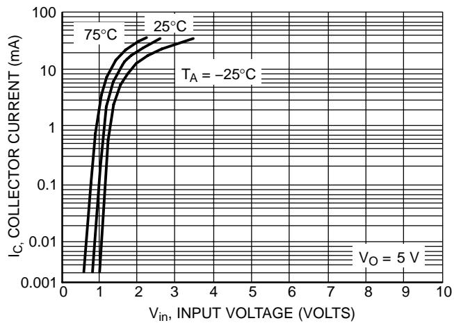
Figure 11. Output Current vs. Input Voltage
