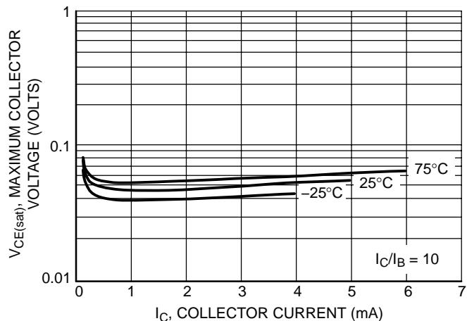
**Figure 33. Maximum Collector Voltage vs. Collector Current**
