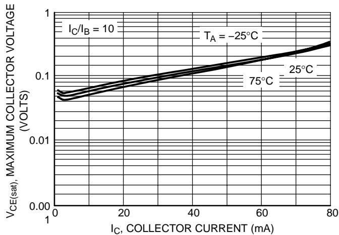
Figure 18.  $V_{CE(\text{sat})}$  vs.  $I_C$
