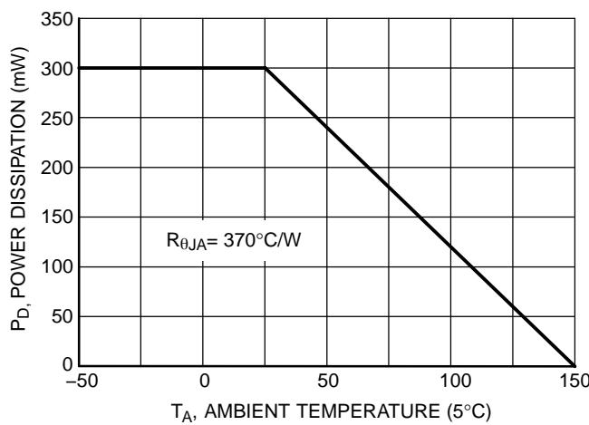
Figure 1. Derating Curve
