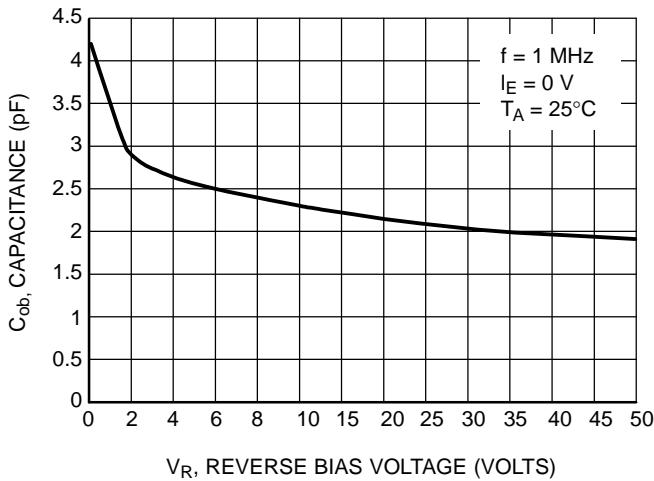
Figure 20. Output Capacitance
