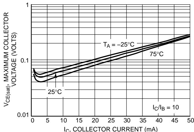
**Figure 38. Maximum Collector Voltage vs. Collector Current**
