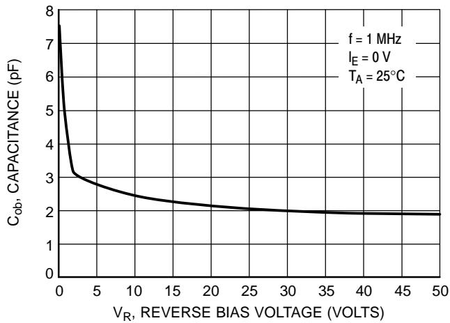
Figure 30. Output Capacitance
