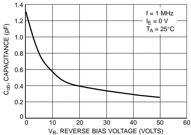
**Figure 40. Output Capacitance**
