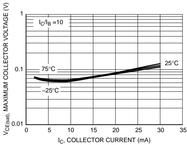
Figure 23.  $V_{CE(\text{sat})}$  vs.  $I_C$
