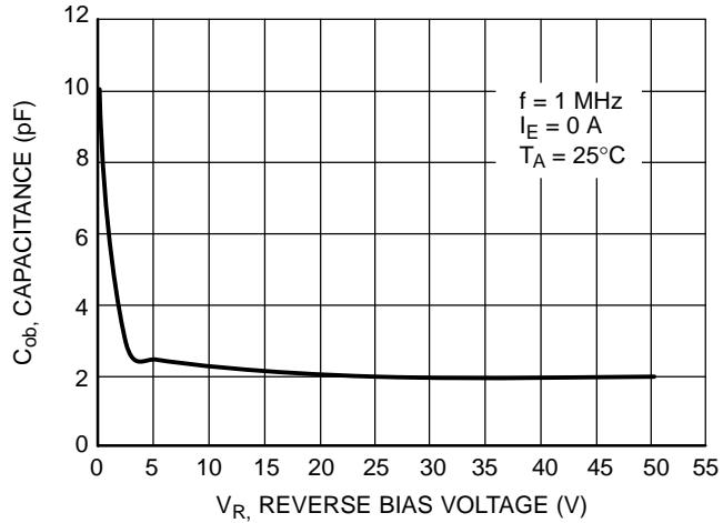
Figure 25. Output Capacitance
