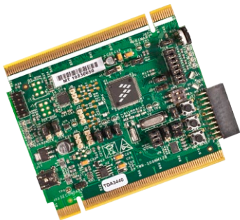
Figure 3: TWR-S08MM128 with Default Jumpers Used in Table 1
