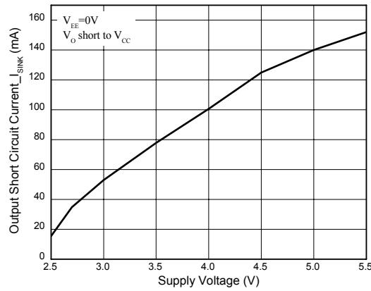
Figure 8. Output Short Circuit Current vs. Supply Voltage
