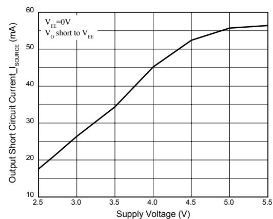
Figure 7. Output Short Circuit Current vs. Supply Voltage
