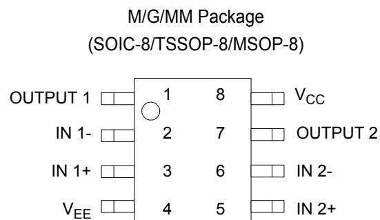
Figure 2. Pin Configuration of AZV358 (Top View)
