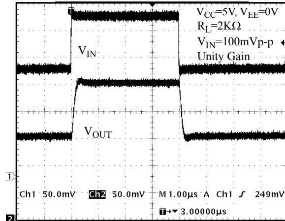
Figure 21. Non-Inverting Input Small Signal Pulse Response
