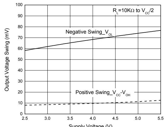
Figure 15. Output Voltage Swing vs. Supply Voltage
