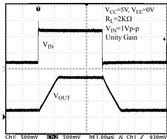
Figure 22. Non-Inverting Input Large Signal Pulse Response
