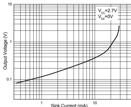
Figure 14. Output Voltage vs. Output Sink Current
