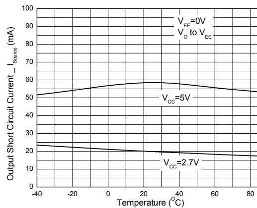
Figure 9. Output Short Circuit Current vs. Temperature
