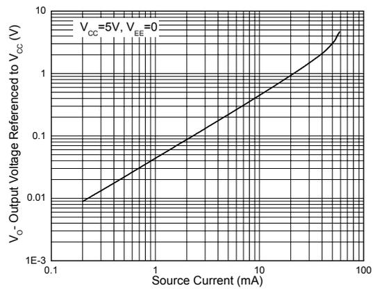
Figure 11. Output Voltage vs. Output Source Current
