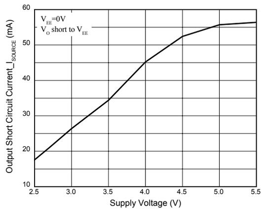
Figure 7. Output Short Circuit Current vs. Supply Voltage
