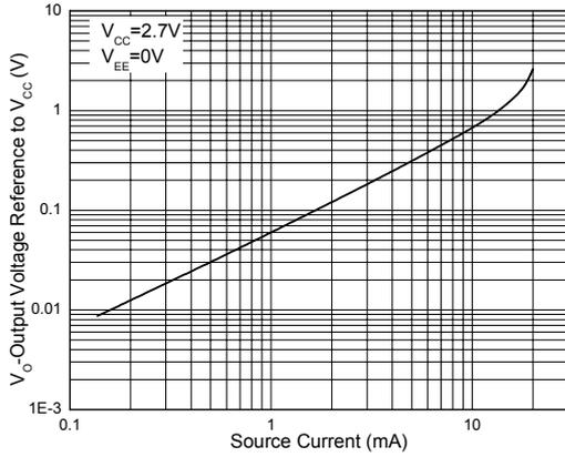
Figure 12. Output Voltage vs. Output Source Current
