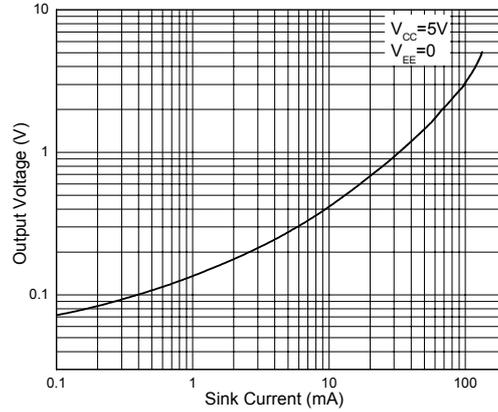
Figure 13. Output Voltage vs. Output Sink Current
