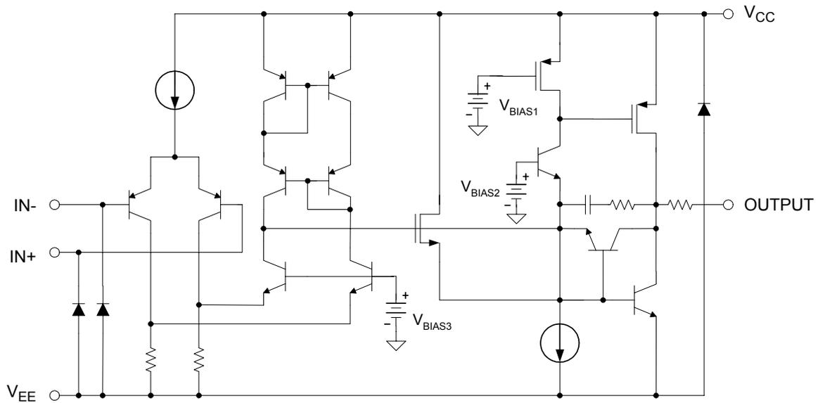
Figure 3. Functional Block Diagram of AZV358 (Each Block)
