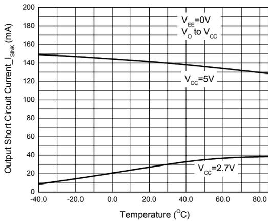
Figure 10. Output Short Circuit Current vs. Temperature
