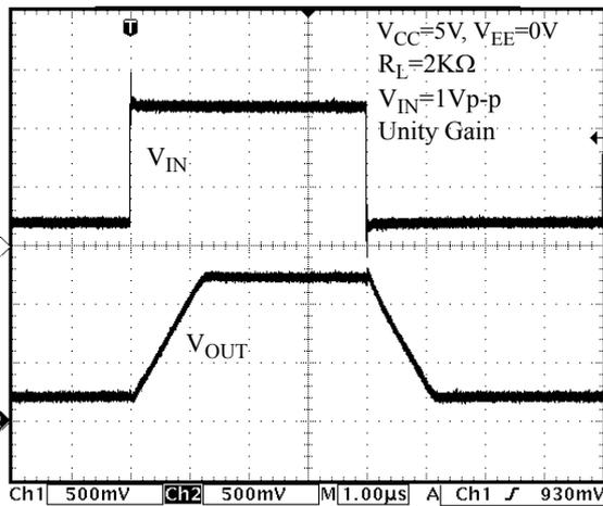
Figure 22. Non-Inverting Input Large Signal Pulse Response
