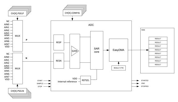
Figure 98: Simplified ADC block diagram
