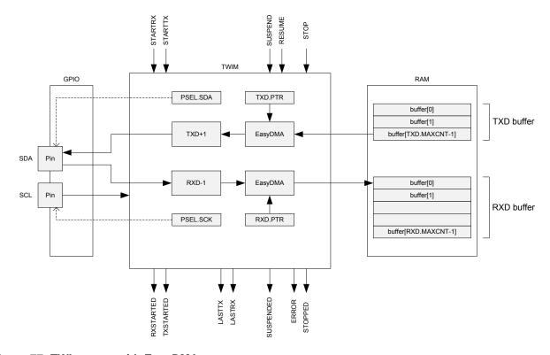
Figure 77: TWI master with EasyDMA
