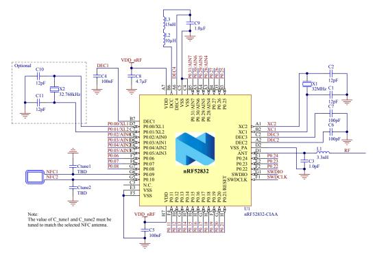
Figure 174: CIAA WLCSP with DC/DC regulator and NFC setup
