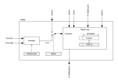
Figure 42: Block schematic for timer/counter
