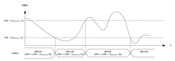
Figure 111: Hysteresis enabled in differential mode
