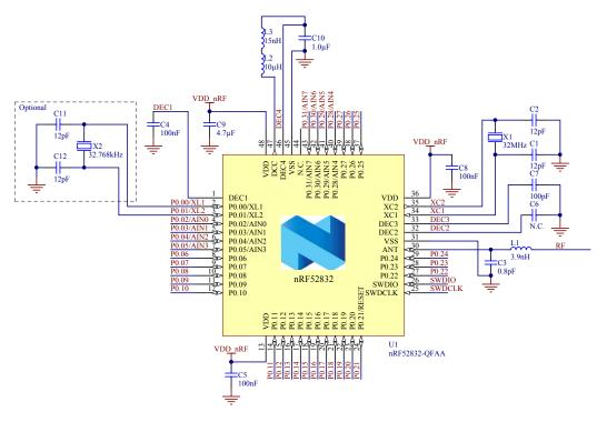
Figure 170: QFAA and QFAB QFN48 with DC/DC regulator setup
