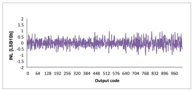
Figure 106: ADC INL vs Output Code
