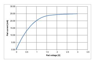
Figure 24: GPIO drive strength vs Voltage, high drive, VDD = 3.0 V
