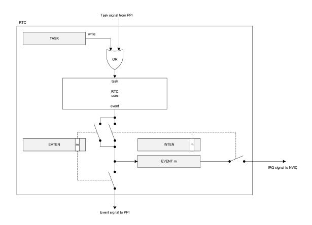
Figure 46: Tasks, events and interrupts in the RTC
