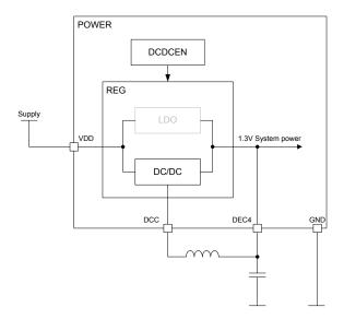
Figure 14: DC/DC regulator setup
