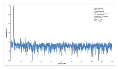
Figure 108: FFT of a 2.8 kHz sine at 200 ksps ()
