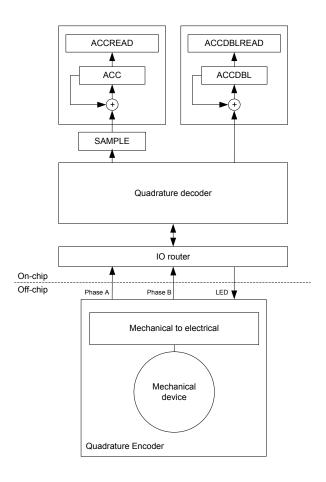
Figure 97: Quadrature decoder configuration
