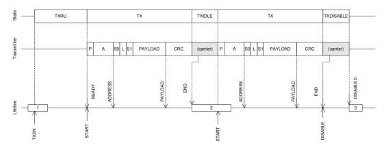
Figure 37: Transmission of multiple packets
