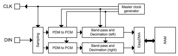
Figure 124: PDM module
