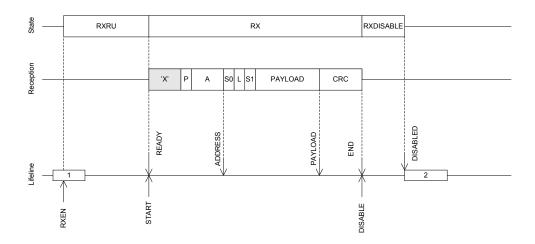
Figure 39: Receive sequence using shortcuts to avoid delays
