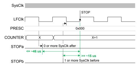
Figure 54: Timing diagram - DELAY\_STOP
