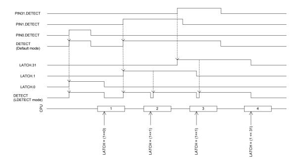
Figure 22: DETECT signal behavior
