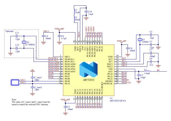
Figure 171: QFAA and QFAB QFN48 with DC/DC regulator and NFC setup
