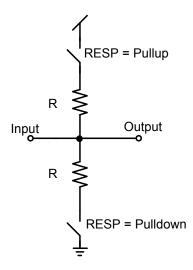
Figure 102: Resistor ladder for positive input (negative input is equivalent, using RESN instead of RESP)
