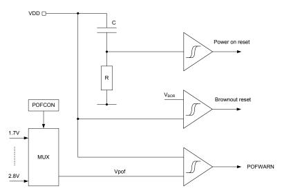
Figure 15: Power supply supervisor
