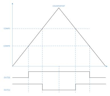
Figure 143: PWM up-and-down counter example
