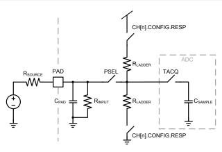
Figure 105: Model of SAADC input (one channel)
