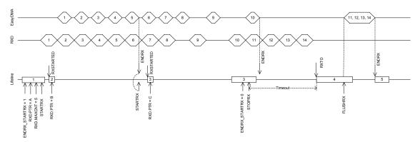
Figure 96: UARTE reception with forced stop via STOPRX
