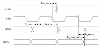
Figure 140: I2S timing diagram
