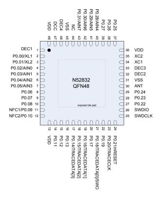
Figure 2: QFN48 pin assignments, top view
