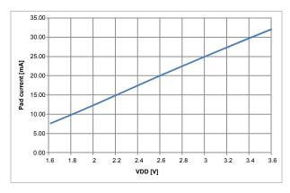
Figure 26: Max sink current vs Voltage, high drive
