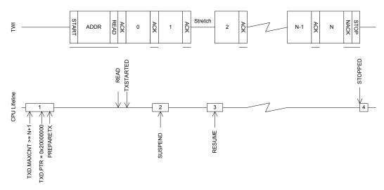
Figure 89: The TWI slave responding to a read command
