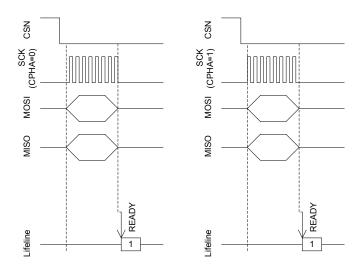
Figure 152: SPI master transaction
