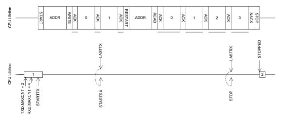
Figure 82: A repeated start sequence, where the TWI master writes two bytes followed by reading 4 bytes from the slave
