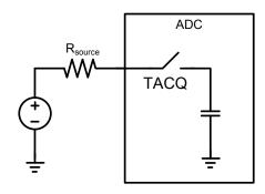
Figure 103: Simplified ADC sample network
