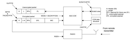
Figure 64: Configuration of on-the-fly decryption
