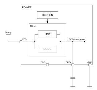
Figure 13: LDO regulator setup
