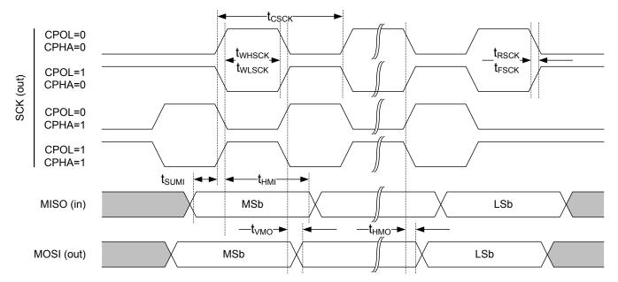
Figure 153: SPI master timing diagram
