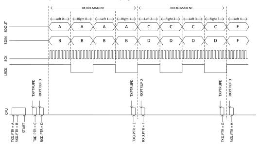
Figure 130: Transmitting and receiving. CONFIG.FORMAT = Aligned, CONFIG.SWIDTH = 8Bit, CONFIG.CHANNELS = Stereo, RXTXD.MAXCNT = 1.
