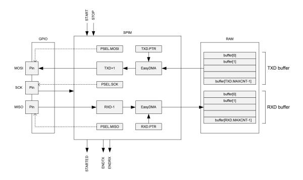
Figure 69: SPIM — SPI master with EasyDMA
