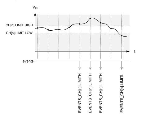
Figure 104: Example of limits monitoring on channel 'n'
