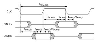
Figure 128: PDM timing diagram
