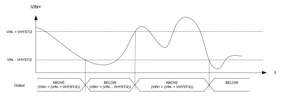
Figure 116: Effect of hysteresis on a noisy input signal
