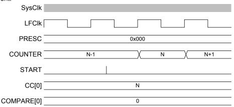
Figure 48: Timing diagram - COMPARE\_START
