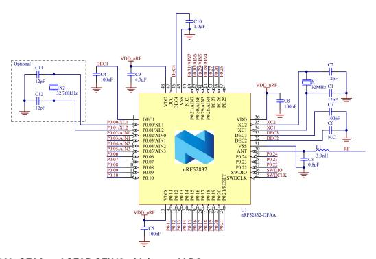
Figure 169: QFAA and QFAB QFN48 with internal LDO setup
