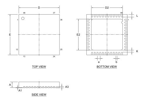
Figure 163: QFN48 6 x 6 mm package
