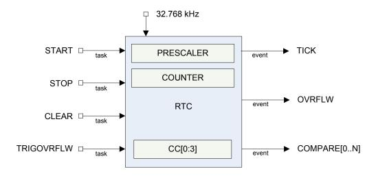
Figure 43: RTC block schematic
