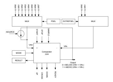
Figure 110: Comparator in differential mode
