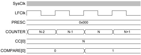
Figure 49: Timing diagram - COMPARE
