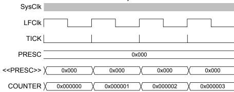
Figure 44: Timing diagram - COUNTER\_PRESCALER\_0
