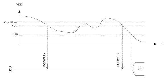
Figure 16: Power-fail comparator (BOR = Brownout reset)
