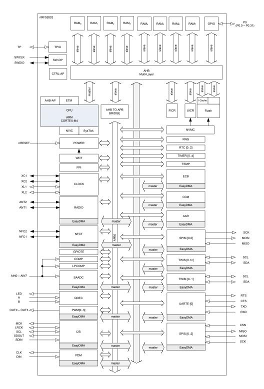
Figure 1: Block diagram
