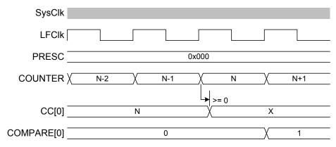
Figure 52: Timing diagram - COMPARE\_N-1
