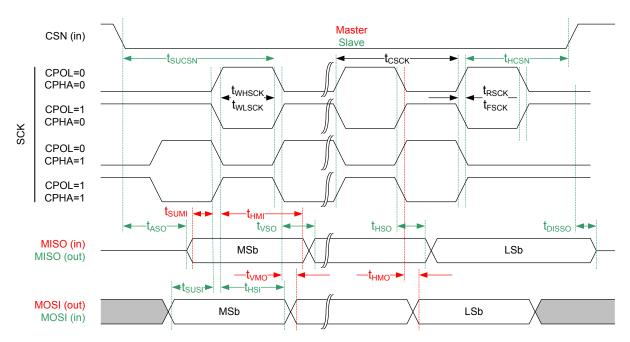
Figure 76: Common SPIM and SPIS timing diagram
