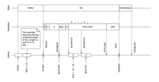
Figure 41: Bit counter example
