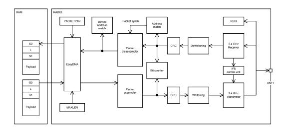
Figure 29: RADIO block diagram
