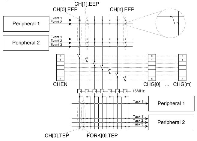
Figure 28: PPI block diagram
