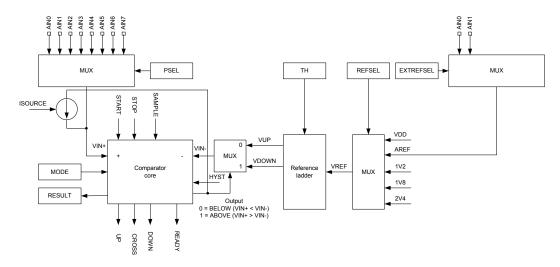
Figure 112: Comparator in single-ended mode
