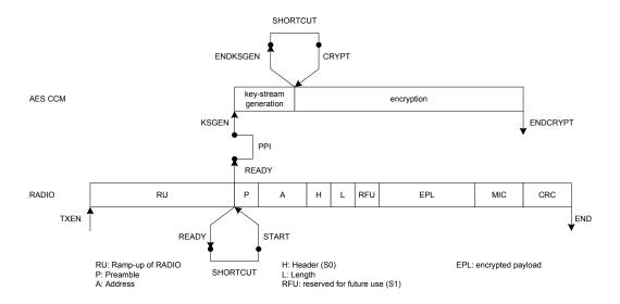
Figure 63: On-the-fly encryption using a PPI connection
