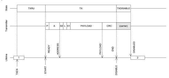
Figure 36: Transmit sequence using shortcuts to avoid delays
