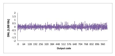
Figure 107: ADC DNL vs Output Code
