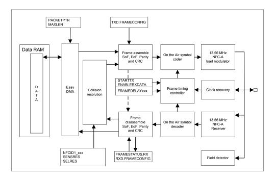
Figure 117: NFC block diagram
