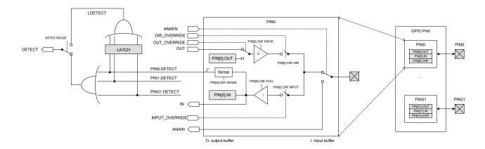
Figure 21: GPIO Port and the GPIO pin details
