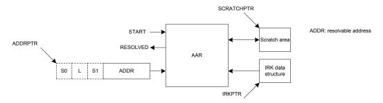
Figure 67: Address resolution with packet preloaded into RAM
