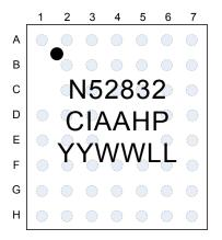
Figure 3: WLCSP ball assignments, top view
