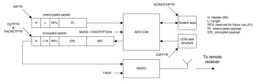
Figure 62: Configuration of on-the-fly encryption
