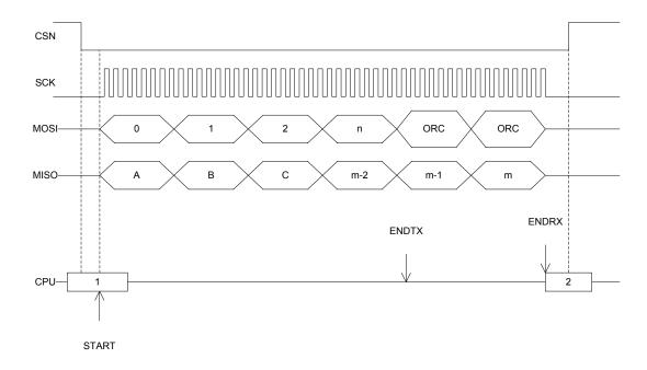
Figure 71: SPI master transaction
