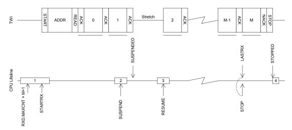
Figure 81: The TWI master reading data from a slave
