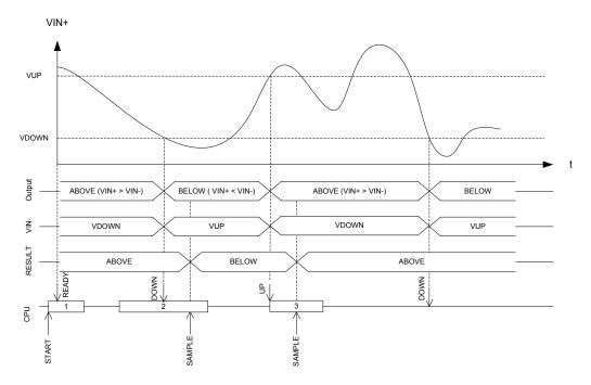
Figure 114: Hysteresis example where VIN+ starts above VUP
