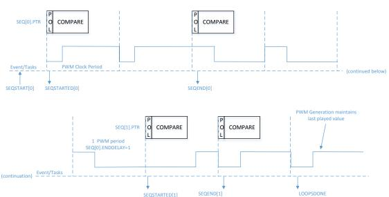
Figure 146: Example using two sequences
