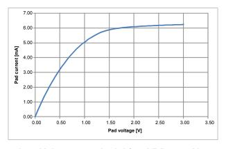
Figure 23: GPIO drive strength vs Voltage, standard drive, VDD = 3.0 V
