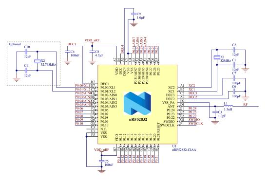
Figure 172: CIAA WLCSP with internal LDO setup
