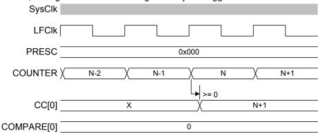
Figure 51: Timing diagram - COMPARE\_N+1
