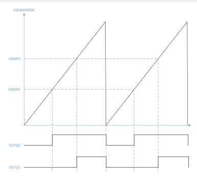
Figure 142: PWM up counter example - FallingEdge polarity
