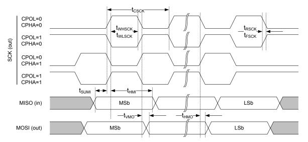
Figure 72: SPIM timing diagram
