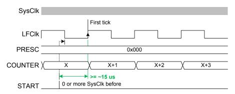
Figure 55: Timing diagram - JITTER\_START-
