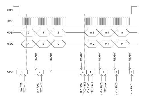
Figure 151: SPI master transaction
