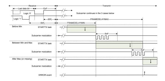
Figure 119: Frame timing controller (FRAMEDELAYMODE=Window)
