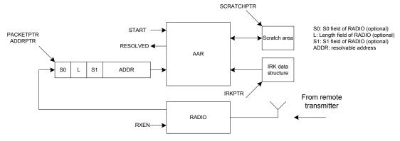
Figure 68: Address resolution with packet loaded into RAM by the RADIO
