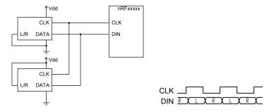
Figure 127: Example of two PDM microphones
