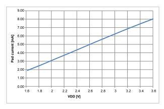
Figure 25: Max sink current vs Voltage, standard drive
