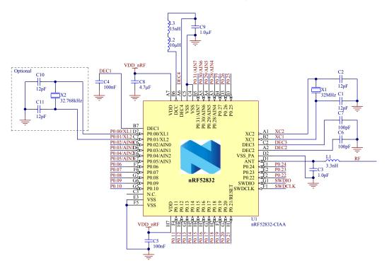
Figure 173: CIAA WLCSP with DC/DC regulator setup
