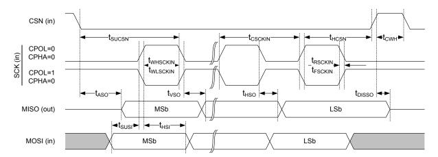
Figure 75: SPIS timing diagram
