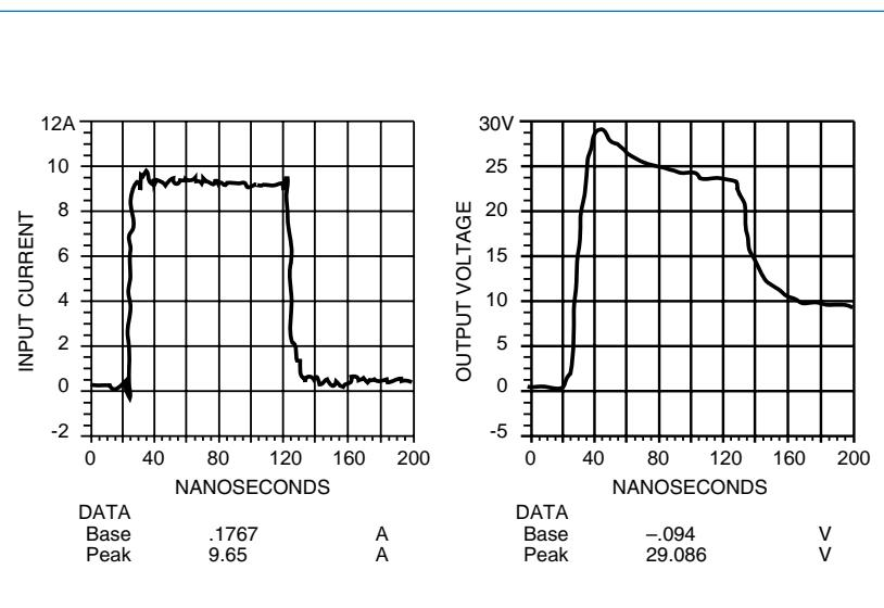
The following chart shows response time and output voltage of a typical MOV with 1000V, 5 nanosecond, 2.5A input pulse mounted in an LJT 13-35P connector. Test was performed without load.
