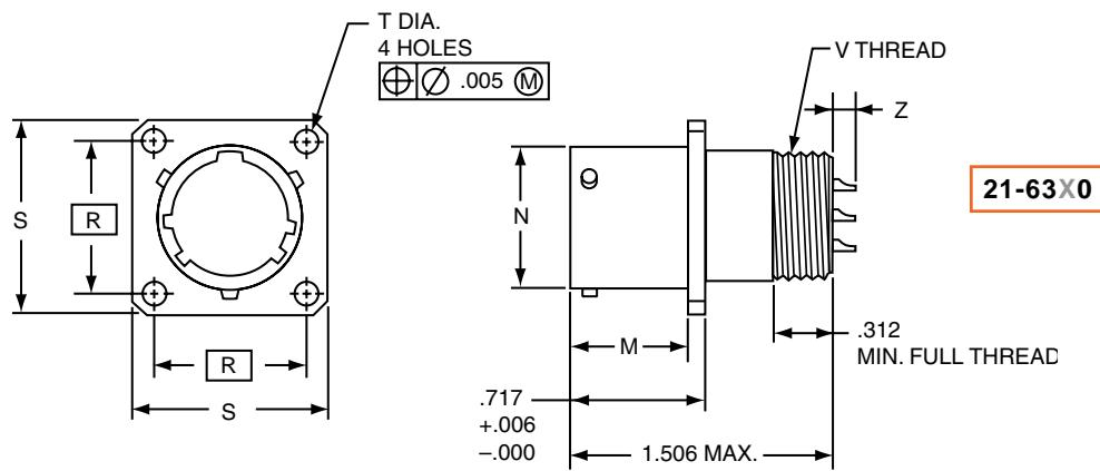
Plug movement required to clear FSJT receptacles: .625 min.
