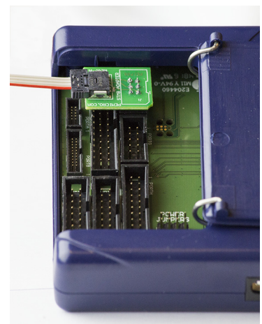
Figure 3-21: STM8 Adapter: 1) Bottom, 2) Top, 3) Connected To 6-Pin Header of Cyclone_Universal (Adapter Sold Separately)
