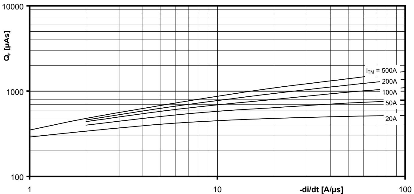
Sperrverzögerungsladung / Recovered charge  $Q_r = f(-di/dt)$  $T_{vj} = T_{vjmax}$ ,  $v_R \leq 0,5 V_{RRM}$ ,  $v_{RM} = 0,8 V_{RRM}$ Parameter: Durchlaßstrom / On-state current  $i_{TM}$
