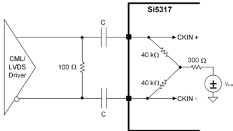
Figure 9. CML/LVDS Termination (1.8, 2.5, 3.3 V)
