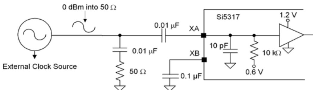
**Figure 15. Sinewave External Reference Clock Input Example**
