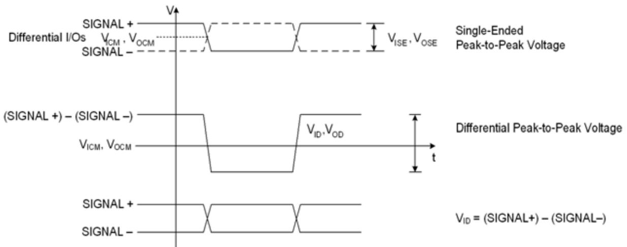
**Figure 1. Voltage Characteristics**
