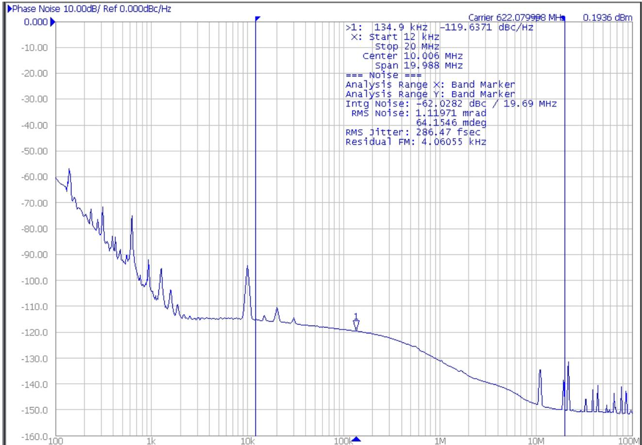
Figure 18. Effect of Reference Frequency on Spurs
