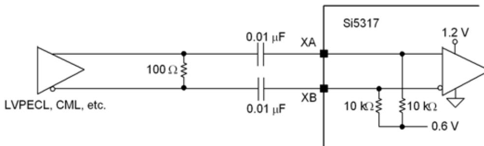
**Figure 16. Differential External Reference Clock Input Example**
