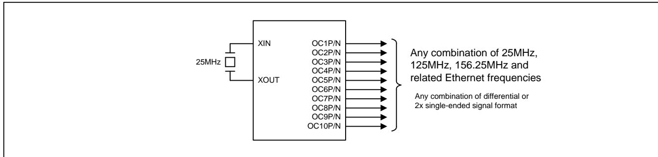
*Figure 1-2. Synchronous Ethernet and SDH/SONET Line Card*
