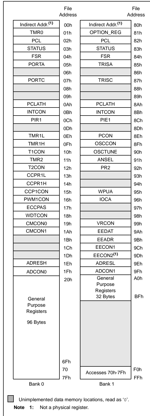
FIGURE 2-2: DATA MEMORY MAP OF THE PIC16F684
