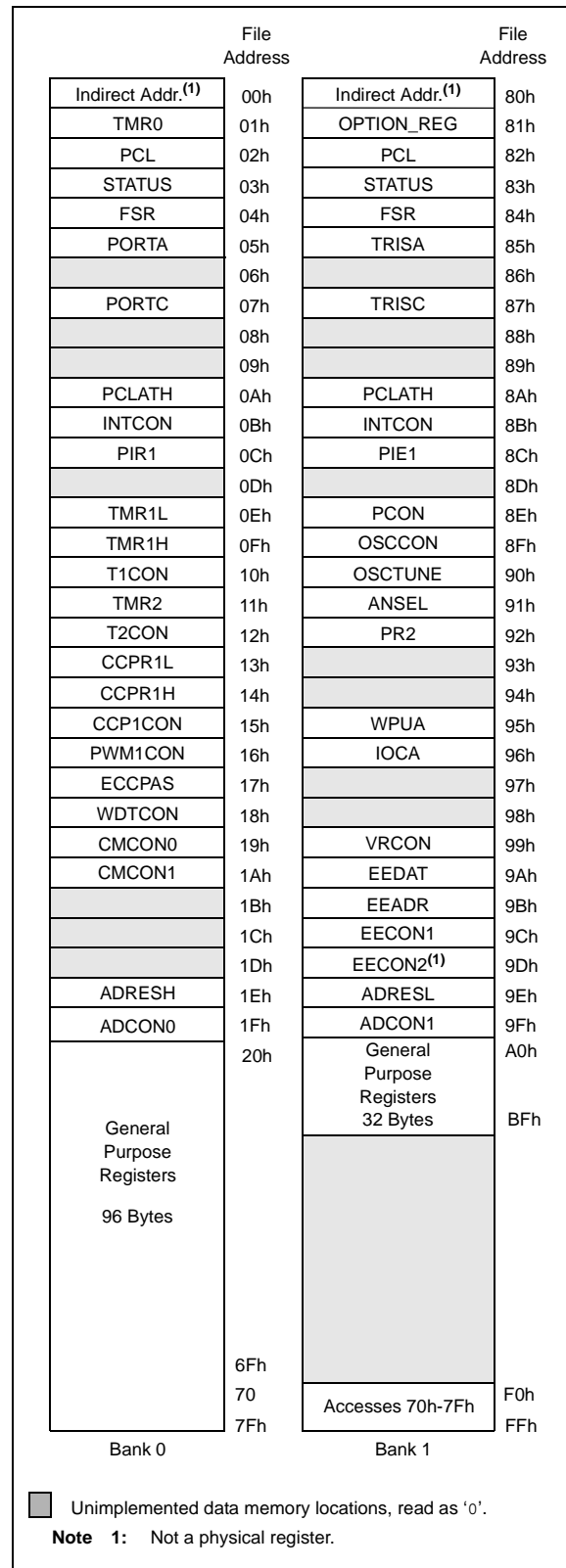
FIGURE 2-2: DATA MEMORY MAP OF THE PIC16F684
