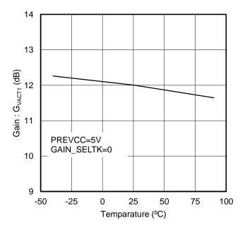
TK Voltage gain 1 (Low gain mode)
