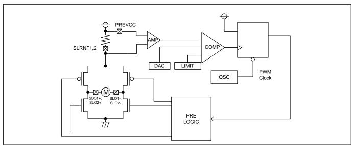
Figure 14. Sled motor driver block
