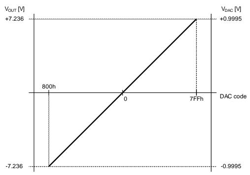
Figure 11. DAC Setting vs. V<sub>DAC</sub> / V<sub>OUT</sub> (in low gain mode)
