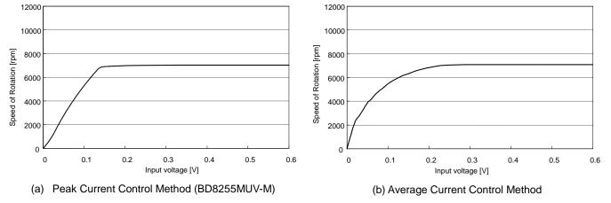
Figure 17. Spindle Driver Input-Output Characteristics
