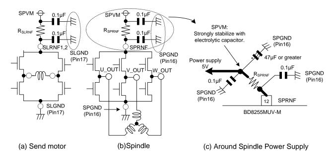
Figure 26. Position of Ceramic Capacitors
