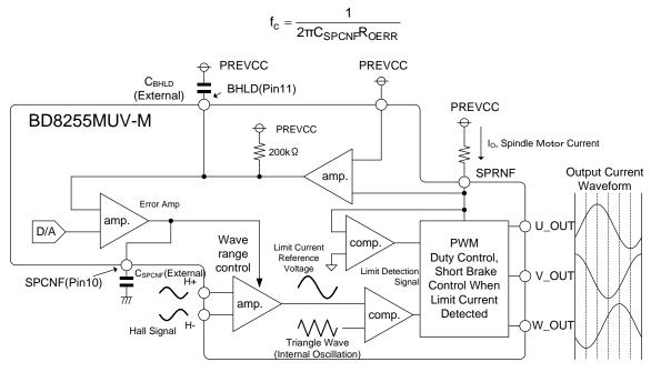
Figure 21. Spindle Driver Block Diagram
