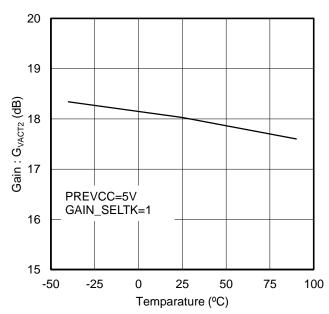
TK Voltage gain 2 (High gain mode)
