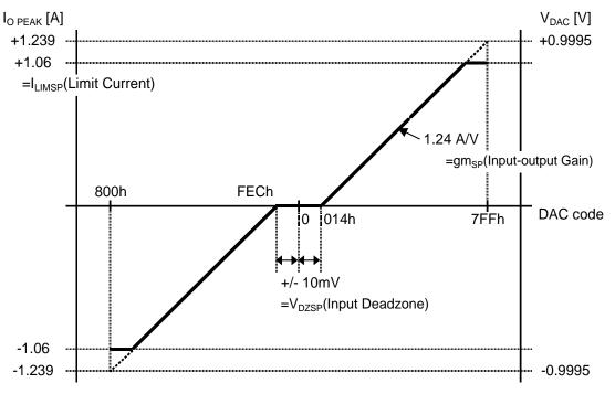
Figure 13.  $I_{O PEAK}$  Characteristics (When set as  $R_{SPRNF}$ =0.33  $\Omega$ ).
