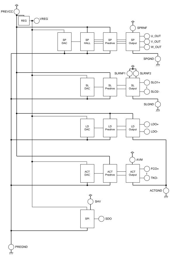
Figure 30. Power Supply and Ground
