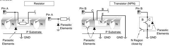
Figure 33. Example of monolithic IC structure
