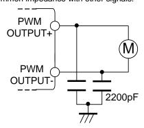
Figure 28. Snubber Circuit
