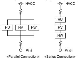
Figure 23. Example of Hall Elements Connection
