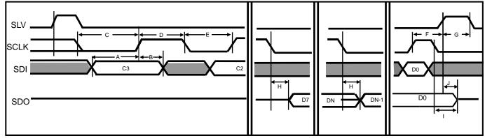
Figure 4. SPI Input / Output Timing
