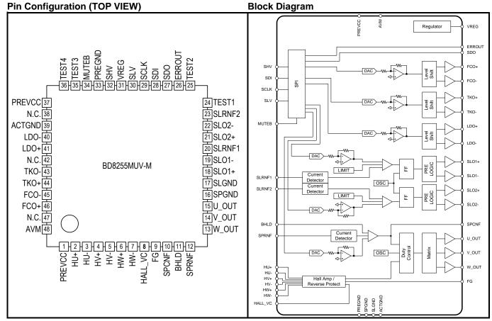
Figure 2. Pin configuration
