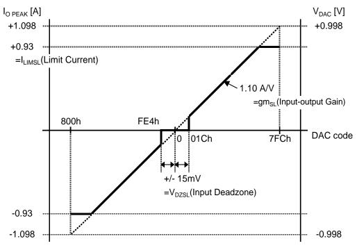
Figure 12.  $I_{O PEAK}$  Characteristics (When set as  $R_{SLRNF}$ =0.56  $\Omega$ ).
