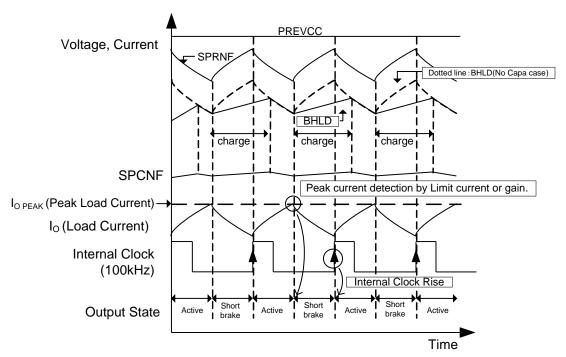
Figure 20. Spindle Driver Operation Timing Chart
