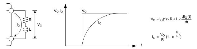
Figure 18. Current Waveform Including Impedance Component
