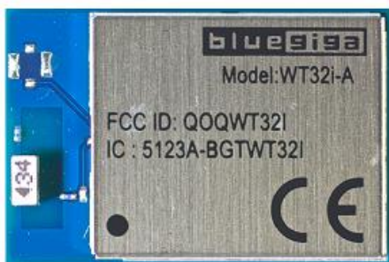
Figure 1: WT32i Bluetooth Audio Module
