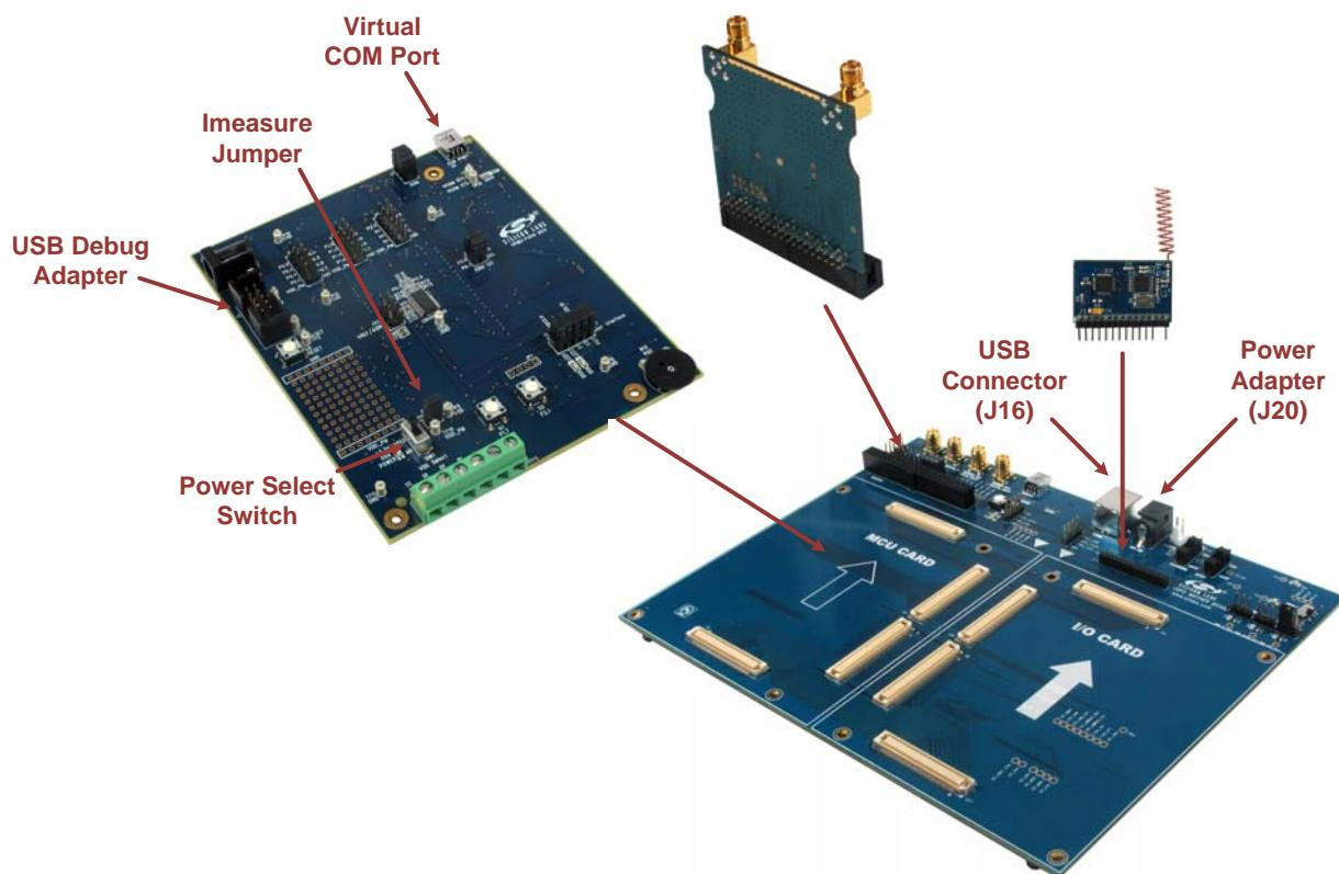
Figure 3. Hardware Setup Using the Unified Development Platform
