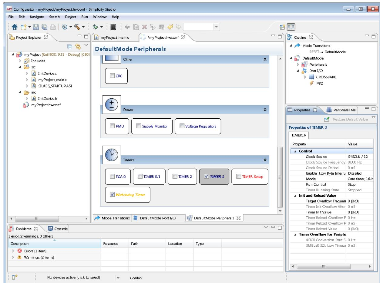
Figure 6. Simplicity Configurator – Configuring Peripheral Properties
