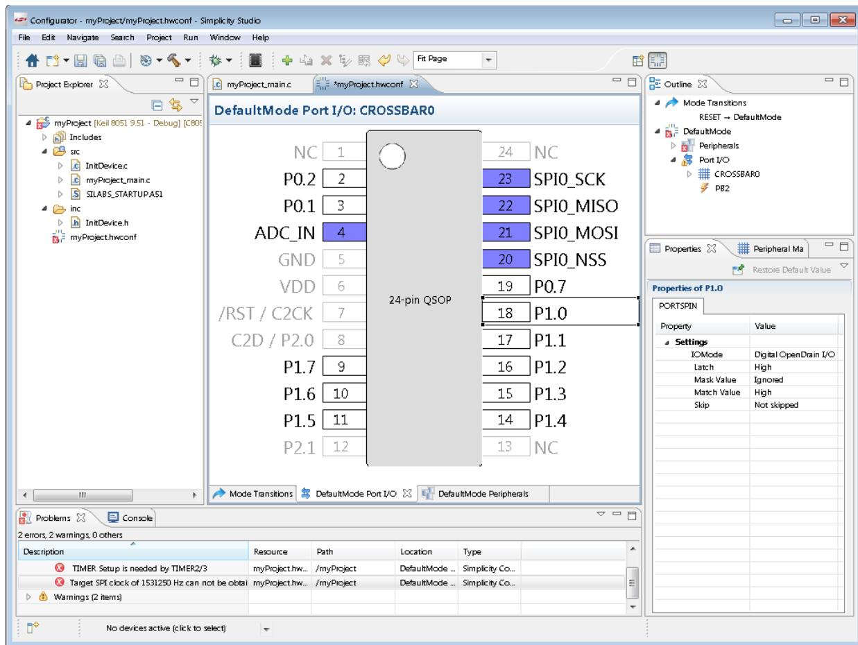
**Figure 7. Simplicity Configurator – Configuring Port I/O**
