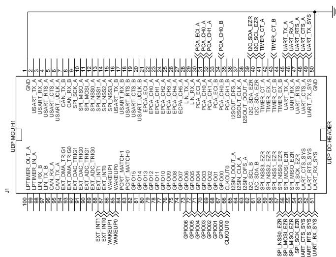
Figure 17. C8051F850 UDP MCU Card Schematic (Revision 200) (4 of 5)
