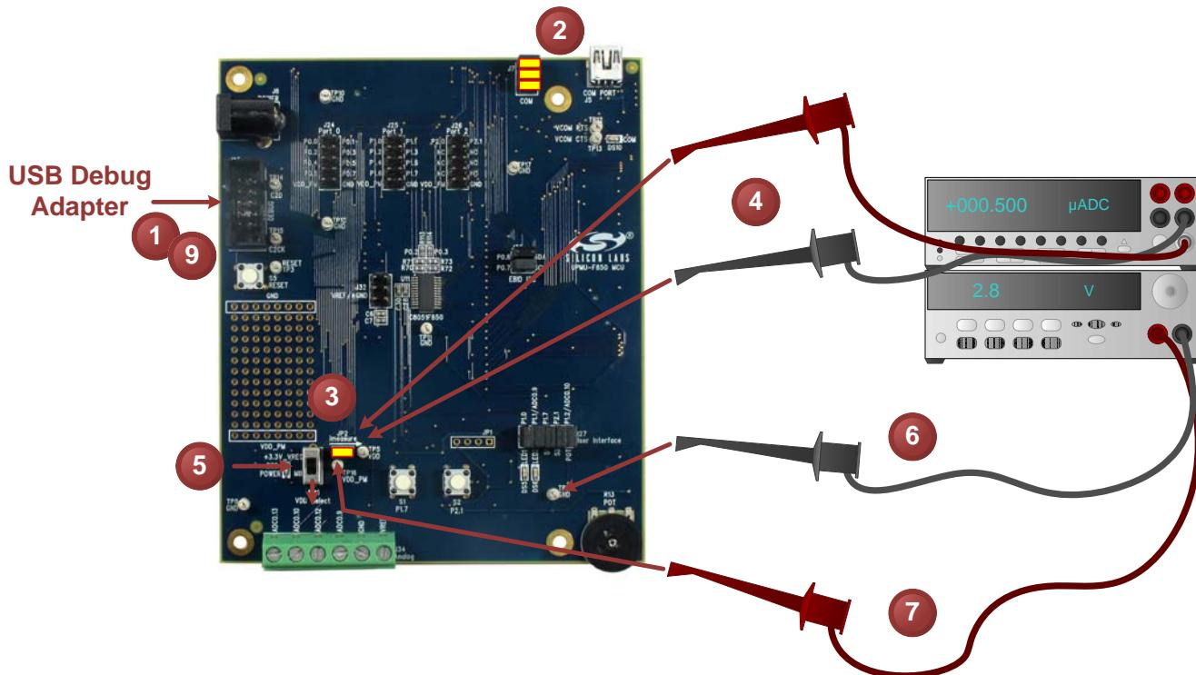
Figure 13. C8051F850 MCU Card Power Measurement Configuration—Varying VDD
