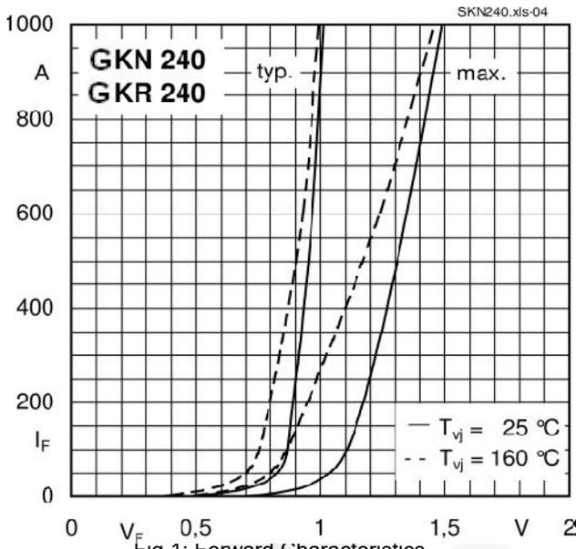
Fig 1: Forward Characteristics
