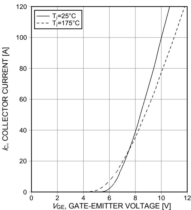
**Figure 7. Typical transfer characteristic**
