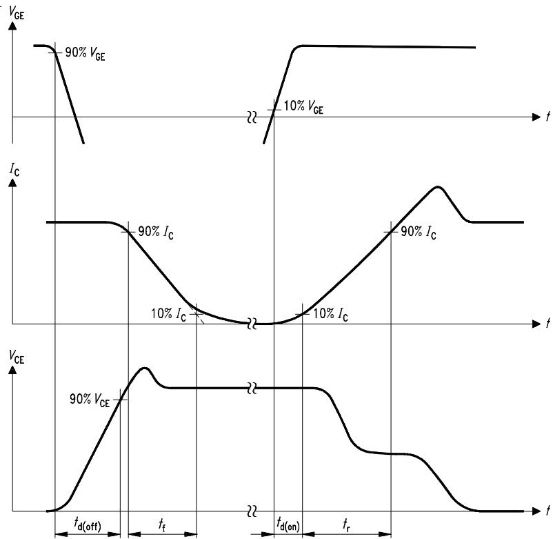
**Figure A. Definition of switching times**
