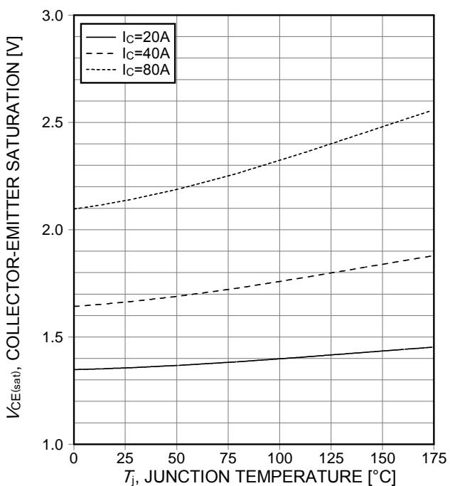
**Figure 8. Typical collector-emitter saturation voltage as a function of junction temperature**
