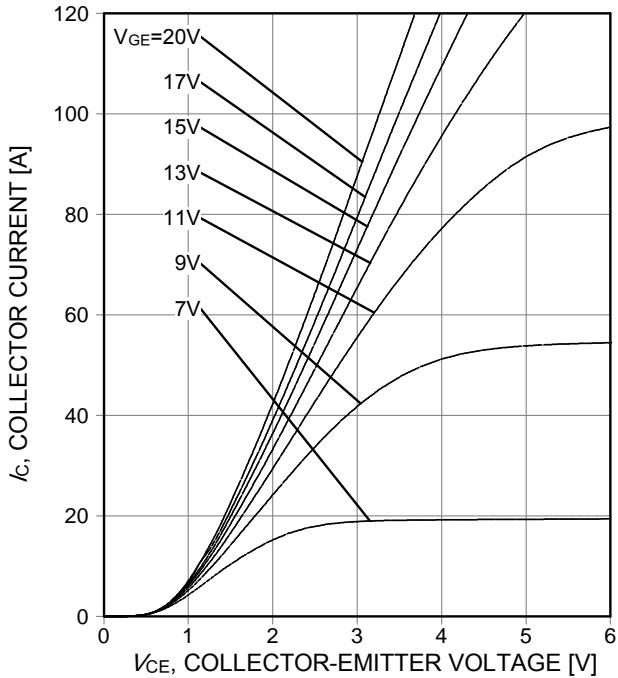
**Figure 6. Typical output characteristic**
