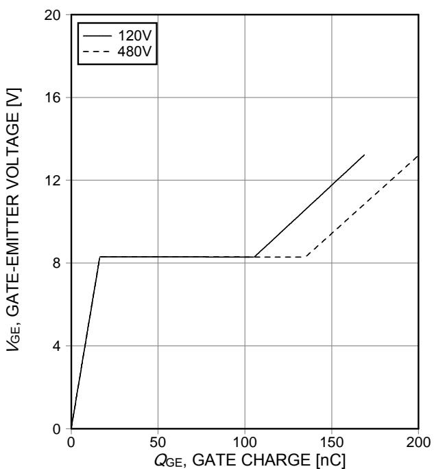
**Figure 16. Typical gate charge**
