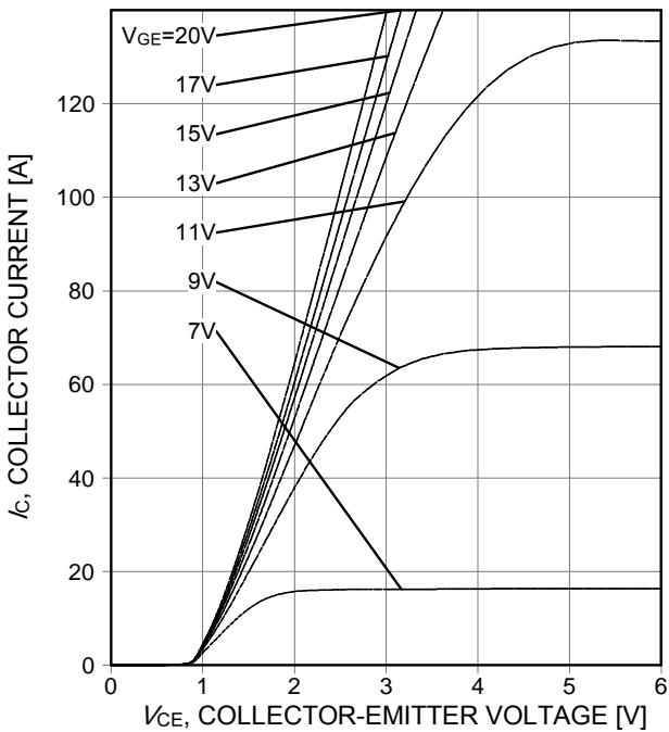
**Figure 5. Typical output characteristic**
