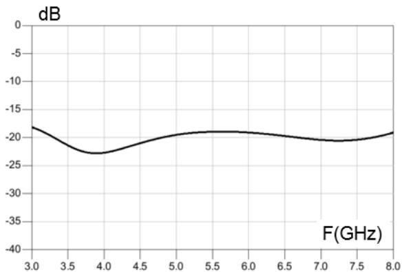
Figure 3. Amplitude imbalance (dB)
