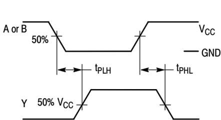
Figure 3. Switching Waveforms
