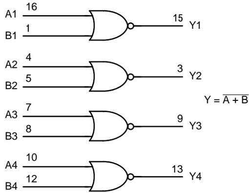
Figure 1. LOGIC DIAGRAM
