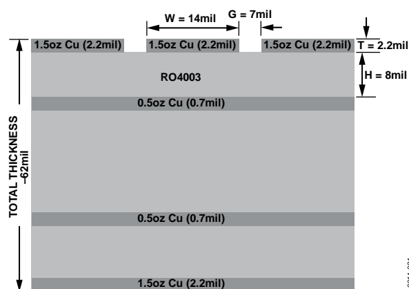
Figure 22. Probe Matrix Board (Cross Section View)
