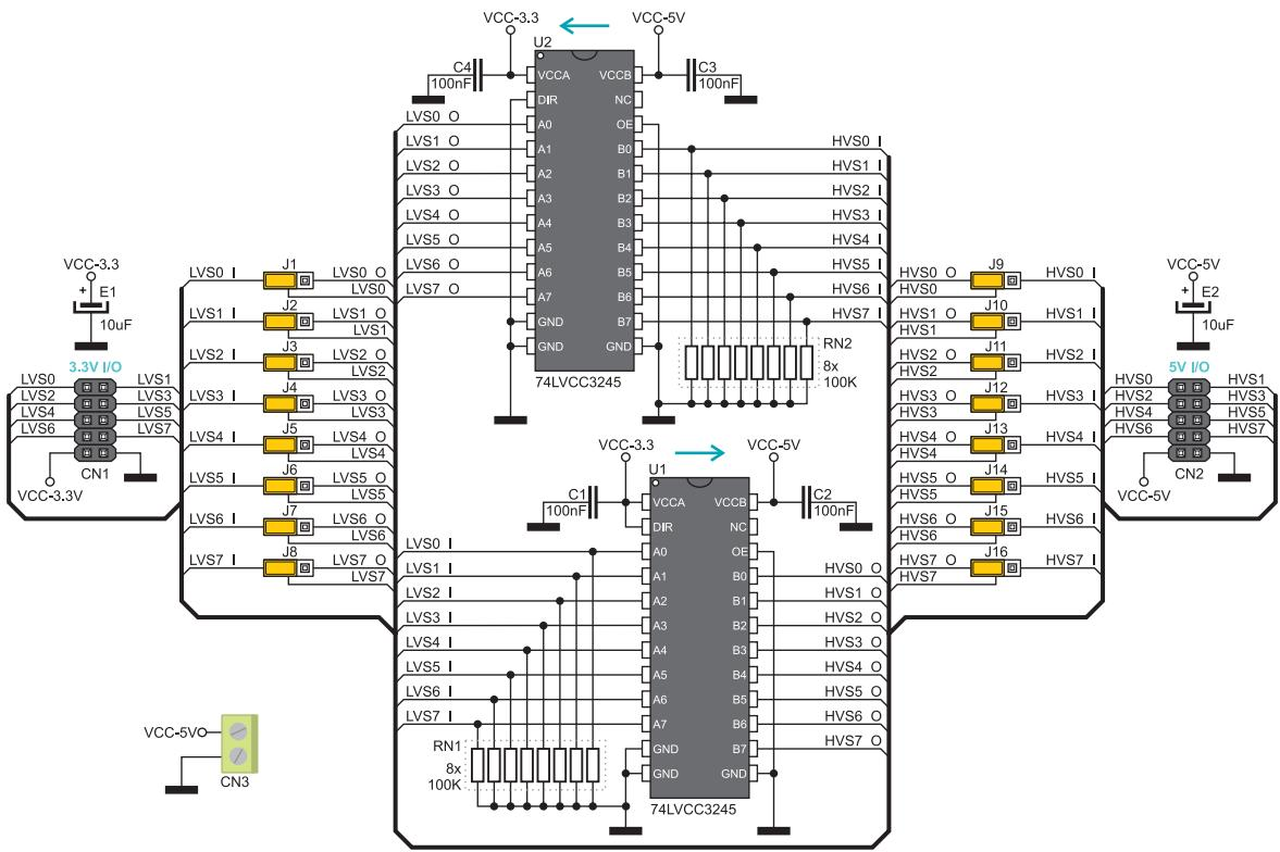
**Figure 6:** 3.3V-5V VOLTAGE TRANSLATOR board connection schematic
