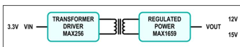
Figure 1. The Riverside subsystem design block diagram.
