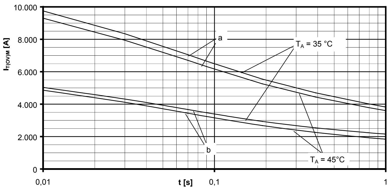
Grenzstrom / Maximum overload on-state current  $I_{T(OV)M} = f(t)$ ,  $v_{RM} = 0,8 \text{ V}_{RRM}$
