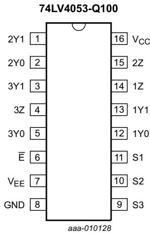
Fig 5. Pin configuration
