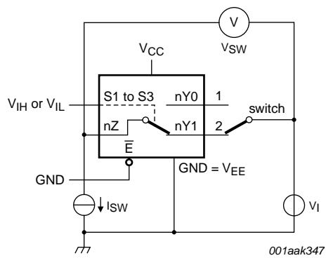
$$R_{ON} = V_{SW} / I_{SW}$$
