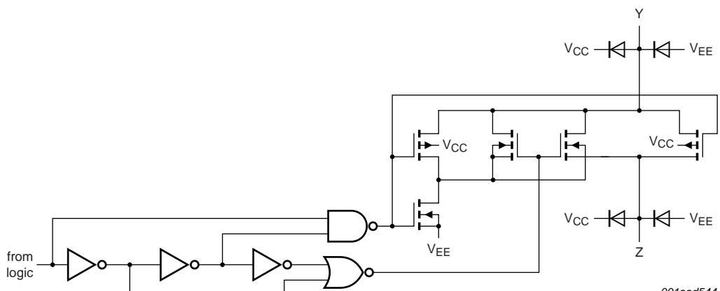
Fig 4. Schematic diagram (one switch)
