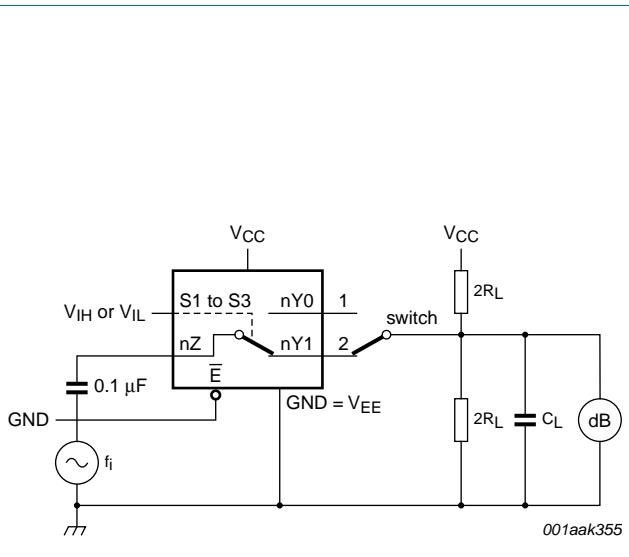
**Fig 16.** Test circuit for measuring frequency response
