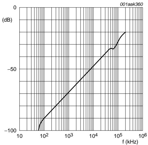
$$V_{CC} = 3.0 \text{ V}; GND = 0 \text{ V}; V_{EE} = -3.0 \text{ V}; R_L = 50 \Omega; R_{\text{SOURCE}} = 1 \text{ k}\Omega.$$
