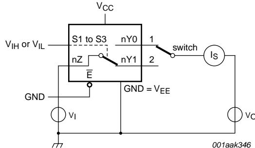
$V_I = V_{CC}$  or  $V_{EE}$  and  $V_O = \text{open circuit}$ .
