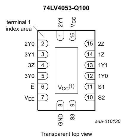
(1) This is not a supply pin. The substrate is attached to this pad using conductive die attach material. There is no electrical or mechanical requirement to solder this pad. However, if it is soldered, the solder land should remain floating or be connected to V<sub>CC</sub>.
