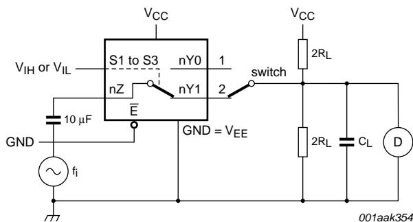
Fig 20. Test circuit for measuring total harmonic distortion
