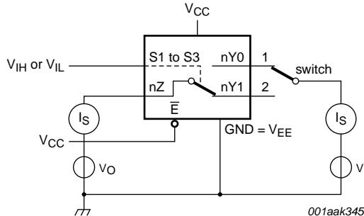
$V_I = V_{CC}$  or  $V_{EE}$  and  $V_O = V_{EE}$  or  $V_{CC}$ .
