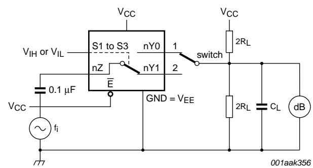
**Fig 18.** Test circuit for measuring isolation (OFF-state)
