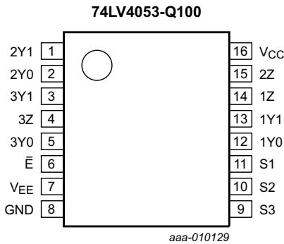
Fig 6. Pin configuration
