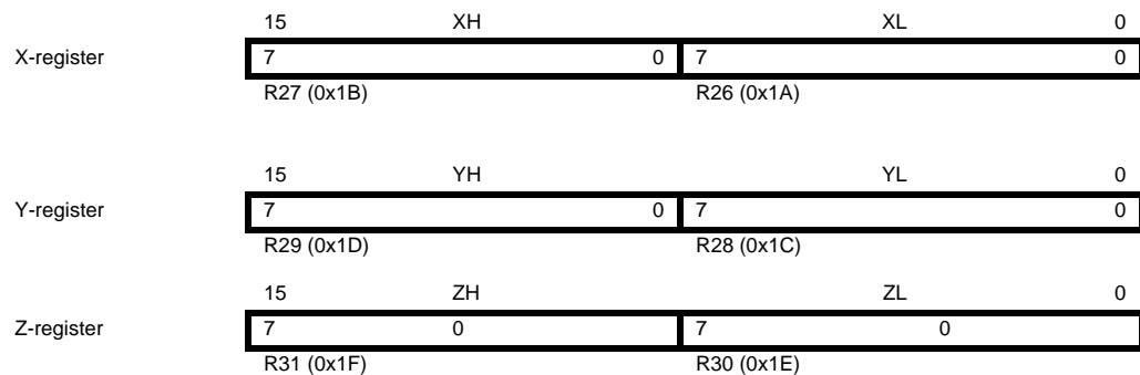
Figure 6-3. The X-, Y-, and Z-registers
