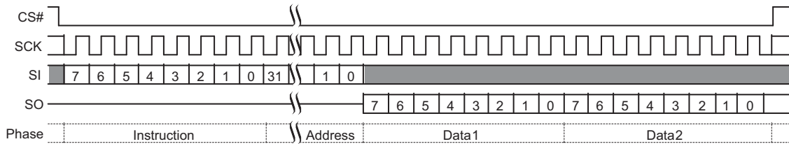
Figure 10. Single Bit Wide I/O Command with Latency
