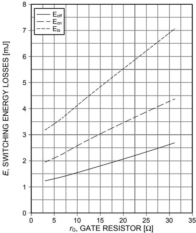
Figure 13. Typical switching energy losses as a function of gate resistor (ind. load,  $T_j=175^\circ\text{C}$ ,  $V_{CE}=400\text{V}$ ,  $V_{GE}=15/0\text{V}$ ,  $I_c=50\text{A}$ , test circuit in Fig. E)
