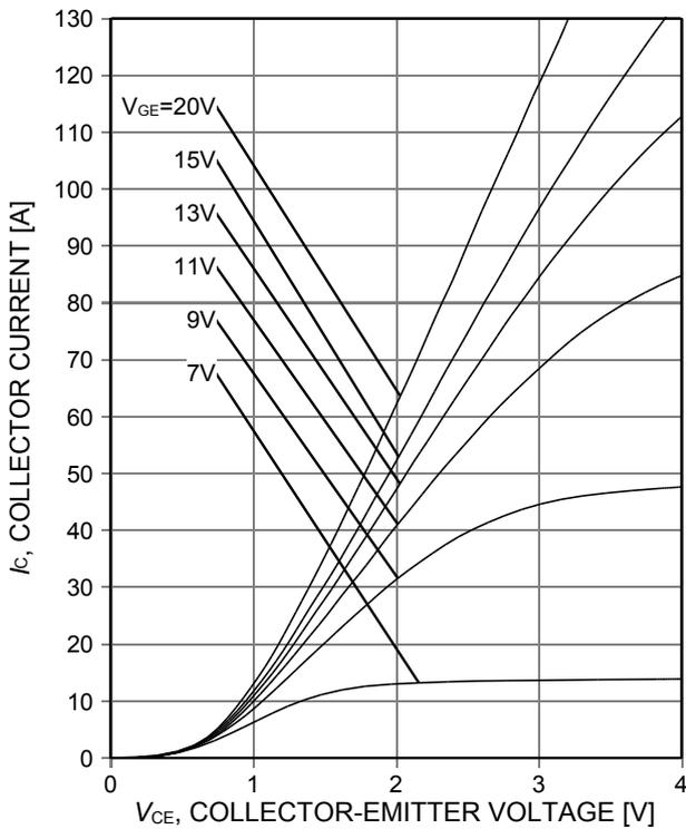
Figure 5. Typical output characteristic ( $T_j=175^\circ\text{C}$ )
