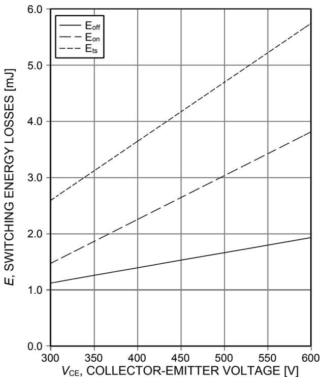
Figure 15. Typical switching energy losses as a function of collector emitter voltage (ind. load,  $T_j=175^\circ\text{C}$ ,  $V_{GE}=15/0\text{V}$ ,  $I_c=50\text{A}$ ,  $r_G=7\Omega$ , test circuit in Fig. E)
