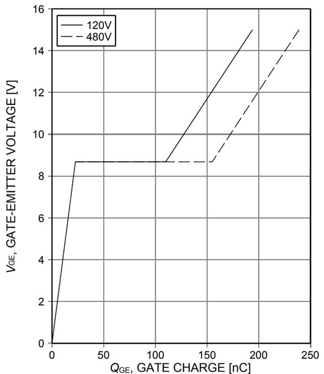
Figure 16. Typical gate charge ( $I_c=50\text{A}$ )
