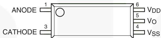
Figure 3. Pin Configuration
