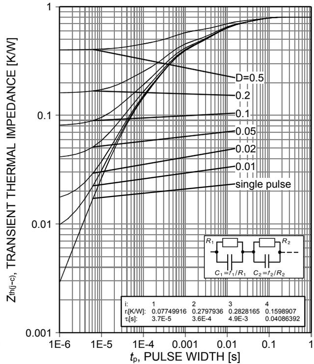
Figure 18. IGBT transient thermal impedance ( $D=t_p/T$ )
