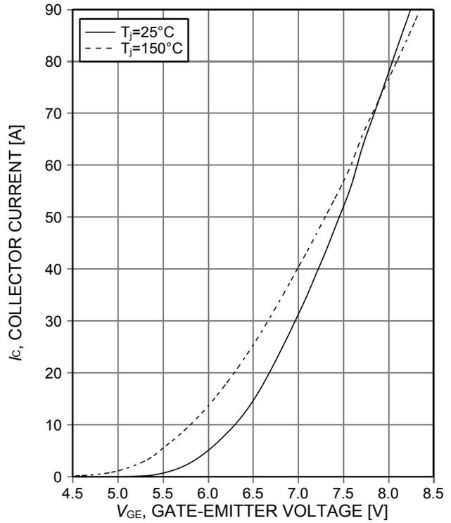
Figure 6. **Typical transfer characteristic**
