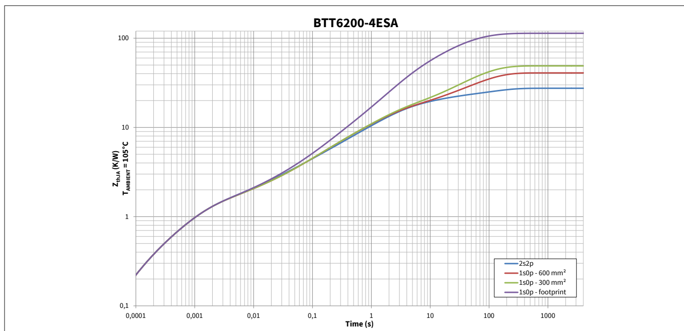
Figure 7 Typical thermal impedance. 2s2p PCB set-up according to Figure 5
