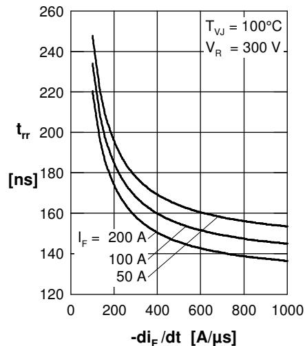
Fig. 5 Typ. recovery time  $t_{rr}$  versus  $-di_F/dt$
