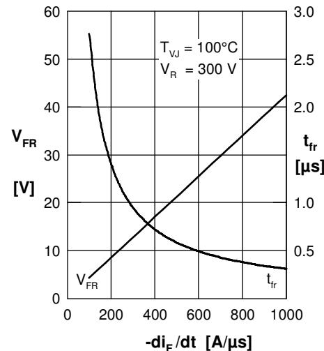
Fig. 6 Typ. peak forward voltage  $V_{FR}$  and  $t_{fr}$  versus  $-di_F/dt$
