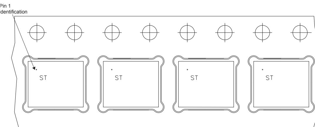
Figure 22. PowerFLAT™ 5x6 reel
