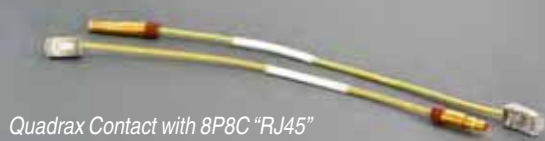
Eight Wire Gigabit Ethernet Assembly
