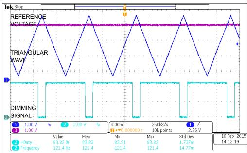
FIGURE 2-5: Obtaining the Dimming Signal - 84% Duty Cycle.
