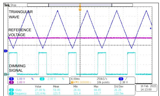
FIGURE 2-6: Obtaining the Dimming Signal - 27%.
