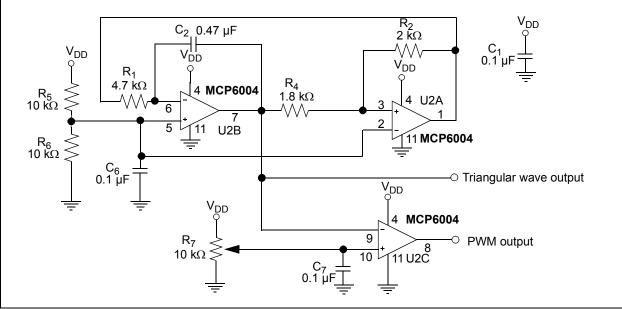
FIGURE 2-4: PWM Dimming Block.
