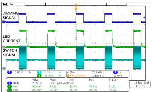
FIGURE 2-7: Dimming Results -  $V_{IN}$  = 4.5V,  $I_{LED\_SET}$  = 90 mA, DUTY = 27%.
