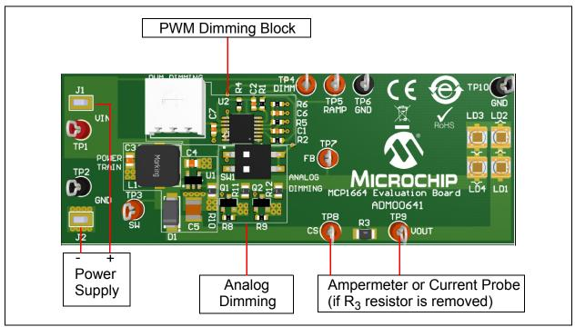
FIGURE 2-2: MCP1664 LED Driver Evaluation Board Setup.
