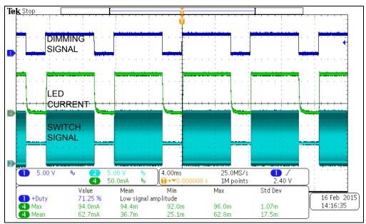
FIGURE 2-8: DIMMING results -  $V_{IN}$  = 4.5V,  $I_{LED\_SET}$  = 90 mA, DUTY = 71%
