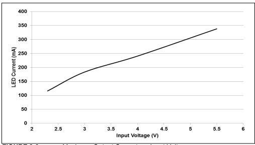
FIGURE 2-3: Maximum Output Current vs. Input Voltage.
